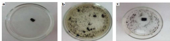
Fig. 5 The recycling of the SWNTs- \beta -CD/PEI-Ad complex. (a) As-prepared sample; (b) The sample was heated in 60 °C water bath; (c) Out of the solvent in the samples and remended the granulates at room temperature.
