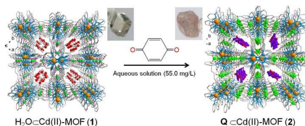
Figure 1. Q adsorption based on 1 in a SC-SC fashion (single-crystal X-ray diffraction indicates that the loaded Q species are disordered in the pores, so only the major disordered components are shown). The single crystal photographs of 1 and 2 are inserted.
