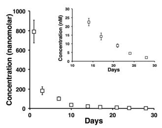
Figure 4 - The 28 day release profile of tritiated vincristine from a 0.5wt% MAX8 peptide hydrogel that initially encapsulated  $10\,\mu\text{M}$  vincristine. After 28 days of release, the amount of drug being released was still in nanomolar quantities, as seen in the inset which highlights days 14 through 28 of the release study.
