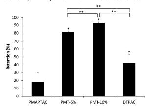
**Fig. 4** Retention of characteristic peaks of antimicrobial coatings after abrasion test. Data represents the standard deviation of three tested samples. *p*-value < 0.05 indicates statistically significant, and \* shows significance between the QAS coated samples and PMAPTAC coated samples, while \*\* shows significance between different QAS coated samples.
