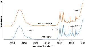
**Fig.2** ATR-FTIR spectra of: (A) PMT-5% copolymer and coating; (B) PMT-10% copolymer and coating.
