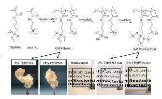
**Fig. 1** Synthesis scheme of QAS copolymers and coatings. The physical appearances of synthesized QAS copolymers of PMT-5% (5% TMSPMA) and PMT-10% (10% TMSPMA) were shown, with the optical transparency of QAS copolymer coatings in comparison to the control.
