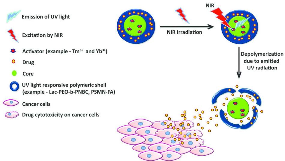
Schematic representation of photoresponsive upconversion nanoparticle showing absorption of NIR by activator followed by emission of UV light which facilitates depolymerization of polymeric sheath and release of drug.
