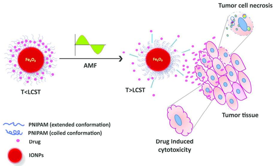
Schematic illustration of NIPAM based AMF responsive nanoparticle showing release of encapsulated drug due to conformational change in polymer from extended to coiled state.
