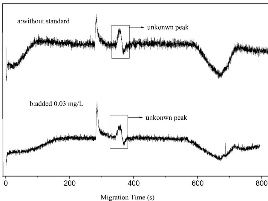
Electropherograms of rays sample (a) and added 0.03mg/L standard herring sample (b)
