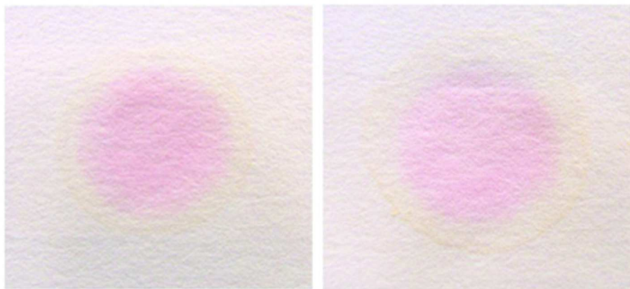
Figure 2 – Spot tests without elution (left) and with elution using two 10 \mu L aliquots of acid buffer (right). 38x18mm (300 x 300 DPI)
