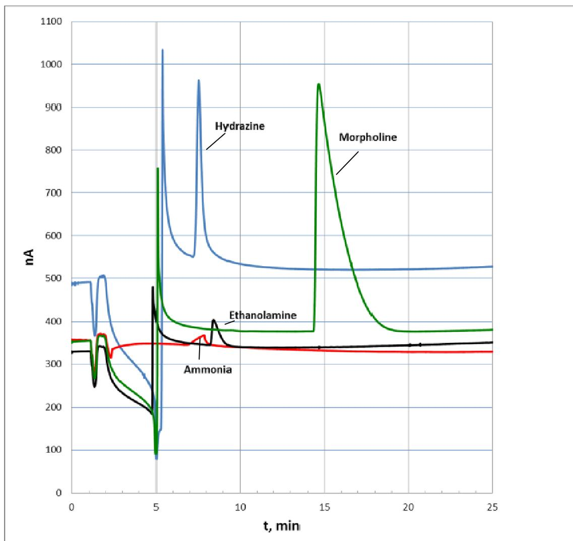
**Figure 4.** Chromatograms of 67  $\mu\text{g/L}$  hydrazine (blue), 300  $\text{mg/L}$  ammonia (red), 300  $\text{mg/L}$  ethanolamine (black) and 300  $\text{mg/L}$  morpholine (green). Column: Zorbax 300-SCX (150x2.1 mm) with a 300-SCX Guard Column (12.5x4.6 mm). Mobile phase: 5  $\text{mmol/L}$  Phosphate buffer (pH 6.0); Flow rate: 0.5  $\text{mL/min}$ ; Amperometric detector in DC mode,  $E=0.8\text{ V}$ .
