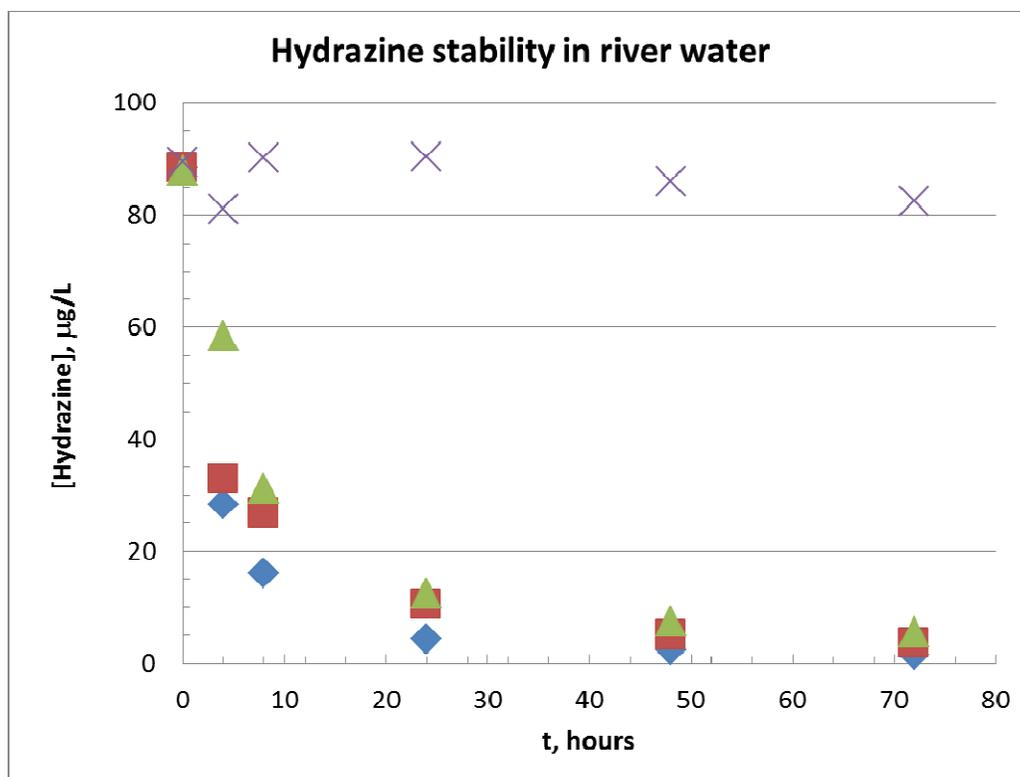
**Figure 7.** The effect of preservation by 10 mmol/L HCl, refrigeration, and ice on hydrazine stability in Rideau River water spiked with 90 µg/L hydrazine over a 3-day period. ◆ - non-preserved; ■ - refrigerated; ▲ - ice; X - 10 mmol/L HCl.
