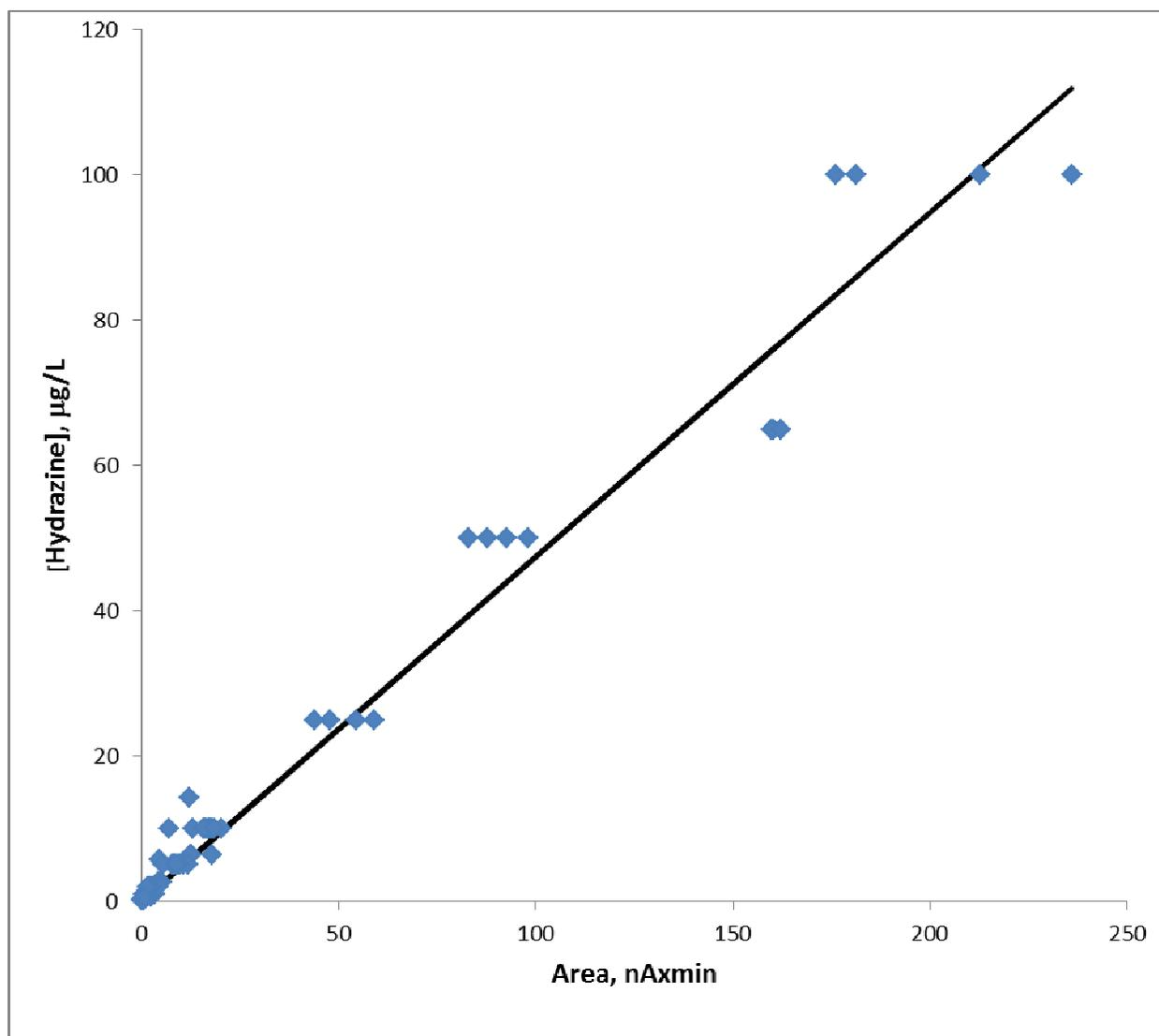
**Figure 5.** Regression analysis of the hydrazine calibration including 82 data points over the period of 6 months by using MS Excel. Multiple R= 0.989;  $R^2= 0.978$ ; observations 82; slope= 0.475; standard deviation= 0.008.
