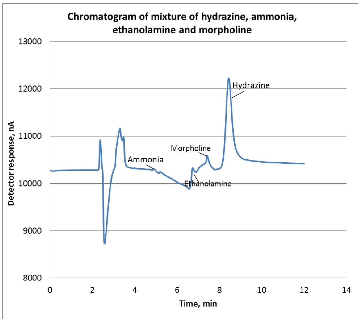
**Figure 3.** A chromatogram of 3 mg/L hydrazine, 400 mg/L ammonia, 400 mg/L ethanolamine and 400 mg/L morpholine. Column: Metrohm C4-250; Mobile phase: 20 % Acetone in 2 mmol/L methanesulfonic acid at a flow rate of 1 mL/min. Amperometric detector in DC mode,  $E = 1.3$  V.
