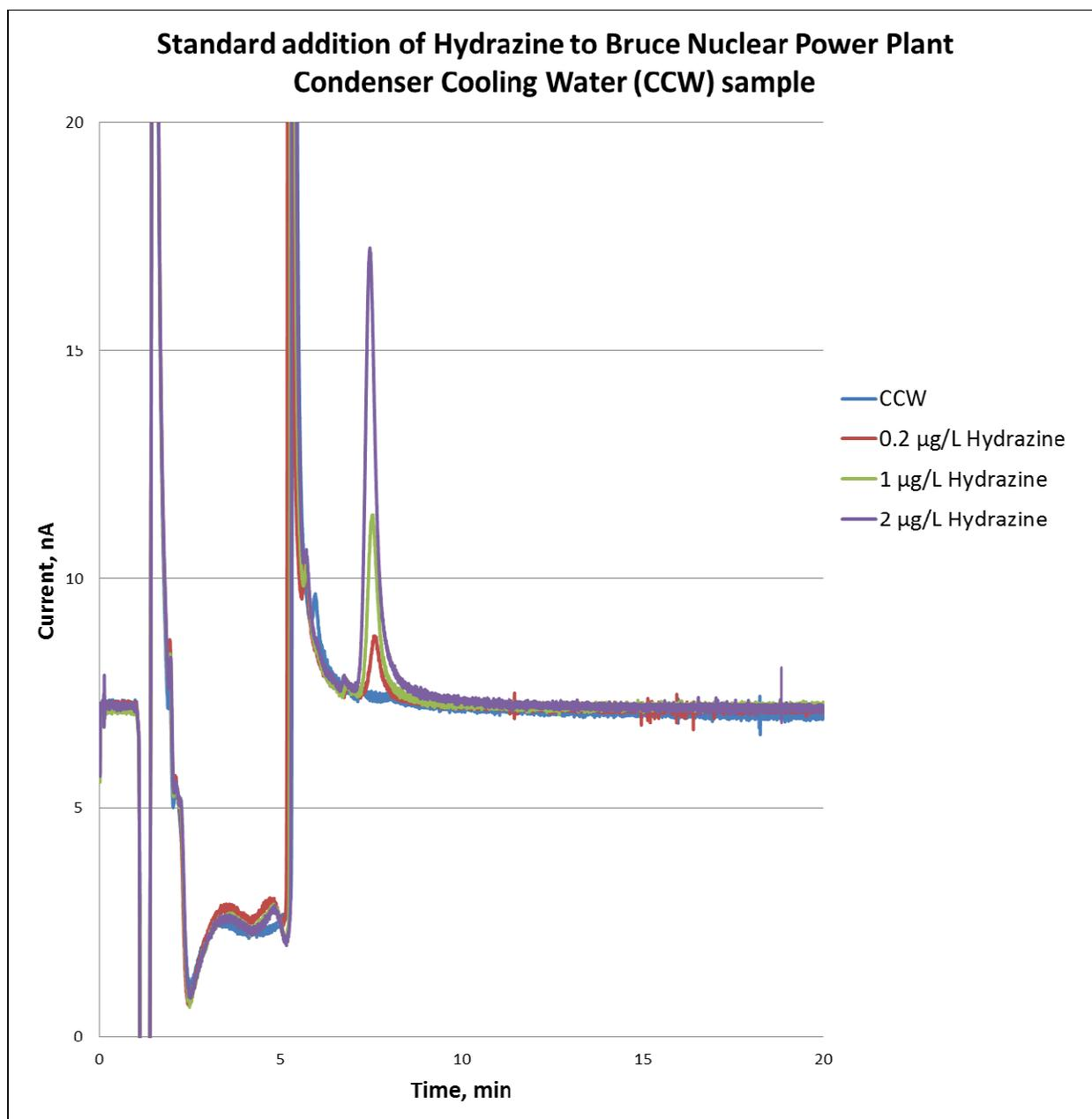
Figure 8. Standard addition method showing the chromatograms of CCW sample, with no hydrazine, and then spiked with 0.2, 1.0 and 2.0 µg/L hydrazine.
