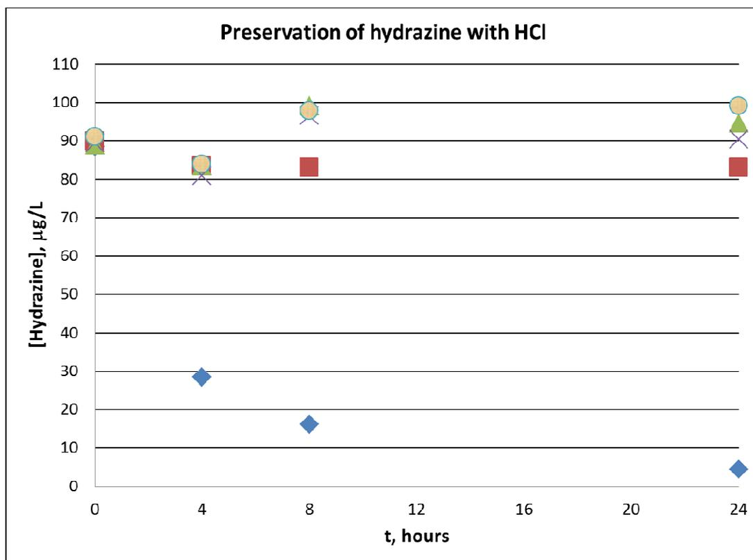
**Figure 6.** The effect of varying concentrations of HCl on hydrazine concentration in Rideau River water sample spiked with 90 µg/L hydrazine.  $\blacklozenge$  – 0 mmol/L HCl;  $\blacksquare$  - 2 mmol/L HCl;  $\blacktriangle$  - 5 mmol/L HCl;  $\times$  – 10 mmol/L HCl;  $\bullet$  - 20 mmol/L HCl.
