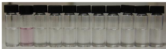
Fig. 4 (a) The absorption spectra and (b) color changes of probe 3 (10 μM) in the mixture of acetonitrile and Tris-HCl buffer (v/v = 9:1, pH = 7.5) after a addition of 200 μM different anions in the form of TBA + salt at 25 °C. From left to right: probe 3, F - , Cl - , Br - , I - , NO 3 - , CN - , ClO 4 - , HSO 4 - , AcO - and H 2 PO 4 - .
