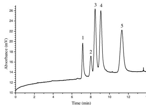
Fig. 5 Chromatograms of thiourea and four aromatic hydrocarbons
