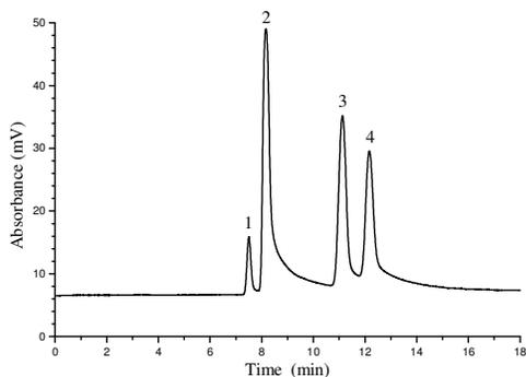
Fig. 7 Electrophoretogram of four neutral compounds
