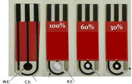
**Figure 1**. Screen-printed electrodes used, indicating in gray the zones of the respective working electrode that were covered during the enzyme immobilization process.
