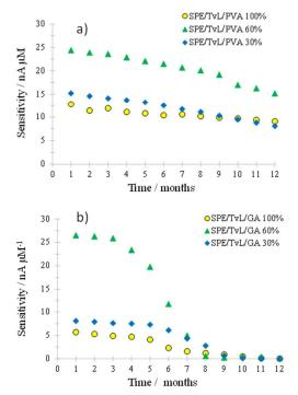
**Figure 3**. Comparison of the sensitivity time variation of a) SPE/TvL/PVA and b) SPE/TvL/GA biosensors: ( $\blacklozenge$ ) towards HQ quantification in acetates' buffer 0.1 M at pH 4.7 ± 0.01 and (30.0 ± 0.5)
