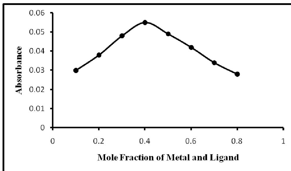
**Fig. 8** Job's method for determination the composition of Se(IV): HNA-OAP (2 : 3) Complex.
