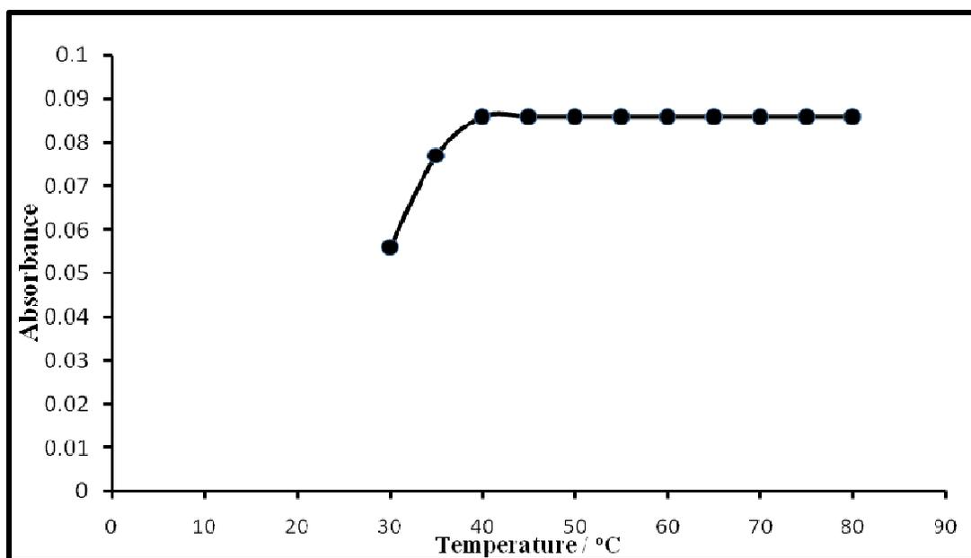
**Fig. 5** Effect of temperature on the Se(IV)-HNA-OAP system.
