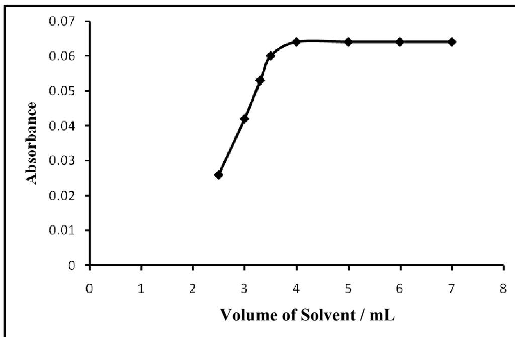
**Fig. 3** Effect of solvent (DMF) on the absorbance of Se(IV)-HNA-OAP system.
