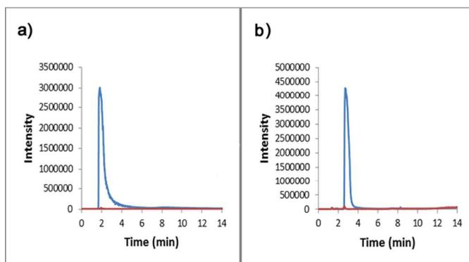
**Figure 3.** Extracted Ion Chromatogram (EIC) of BMPyr-Tf<sub>2</sub>N before (blue) and after (red) SPE in the positive (a) and negative (b) MS mode.
