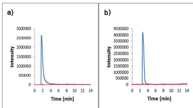
**Figure 2.** Extracted Ion Chromatograms (EIC) of DMPI-Tf<sub>2</sub>N before (blue) and after (red) SPE in the positive (a) and negative (b) MS mode.
