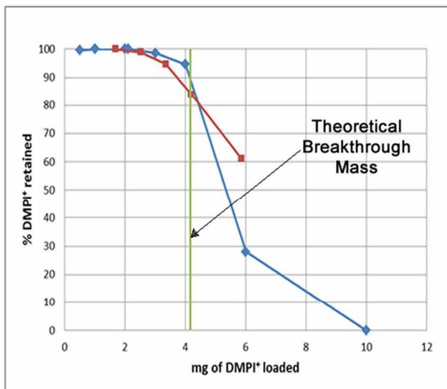
**Figure 4.** Retention of DMPI<sup>+</sup> on the Strata-XC SPE column: (◆) ionic liquid only, (■) ionic liquid with 8.0 wt% tetramethylammonium hydroxide.
