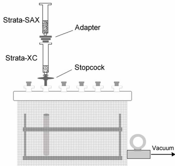
**Figure 1.** SPE column assembly with SPE vacuum manifold.
