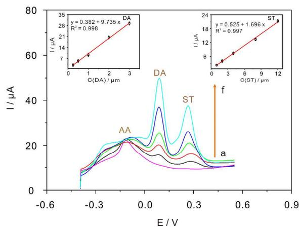
**Fig. 7** DPV responses of PCA/ACPE to AA, DA and ST mixed in the buffer of 0.1 M PBS (pH 7.4).  $c(\text{AA}) = 50$   $\mu\text{M}$ ;  $c(\text{DA})$  (a→f): 0, 0.25, 0.5, 1, 2 and 3  $\mu\text{M}$ ;  $c(\text{ST})$  (a→f): 0, 1, 2, 4, 8 and 12  $\mu\text{M}$ ; Pulse amplitude = 50 mV, pulse width = 50 ms, sample width = 40 ms and pulse period = 100 ms.
