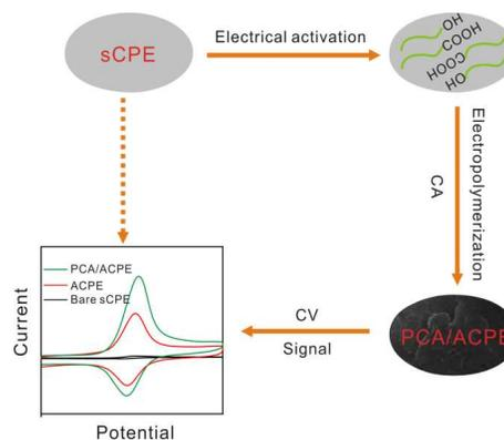
**Scheme 1** Schematic illustration of strategy for the detection of DA and ST based on electrodeposition of CA on ACPE.
