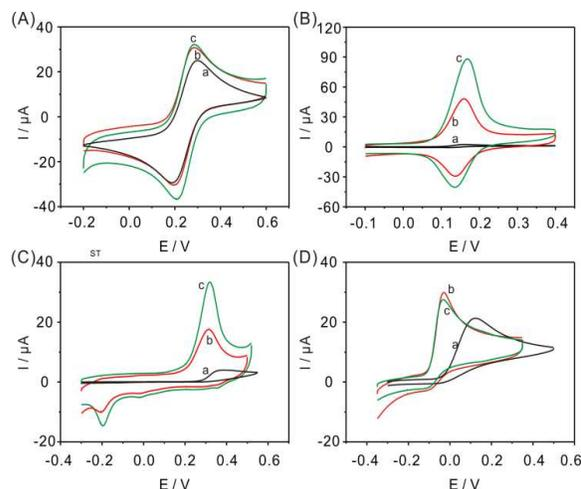
**Fig. 4** CVs obtained in 1.0 mM  $[\text{Fe}(\text{CN})_6]^{3-/4-} + 1.0 \text{ M KCl}$  (A), and in 0.1 M pH 7.4 PBS containing 0.1 mM of DA (B), ST (C), or AA (D), using CPE (a), ACPE (b) and CA/ACPE (c). Scan rate  $50 \text{ mV} \cdot \text{s}^{-1}$ .
