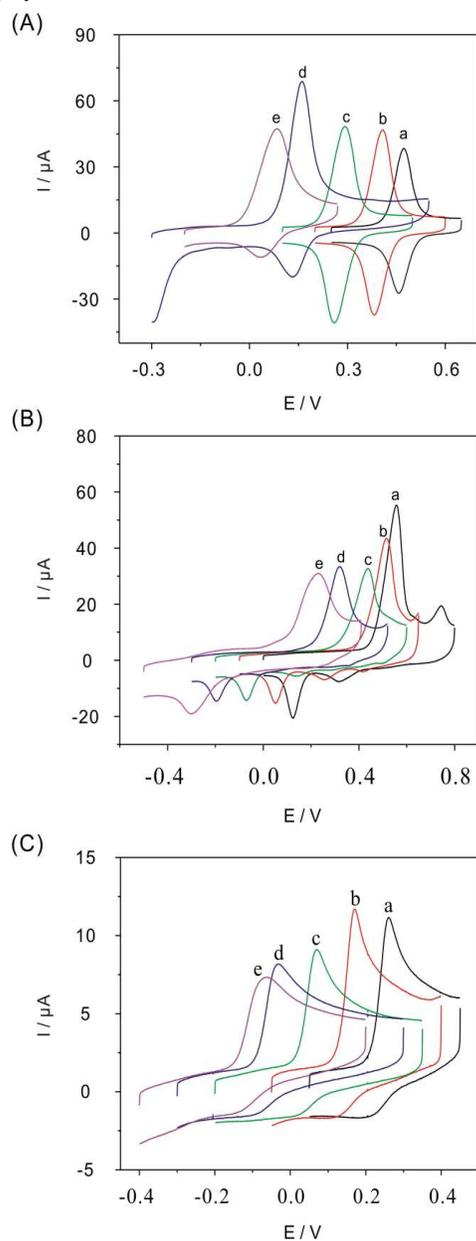
**Fig. 3** CVs at CA/ACPE in (A) 0.1 mM DA, (B) 0.1 mM ST and (C) 0.1 mM AA with different pHs. (a→e): 2.0, 3.3, 5.3, 7.4 and 9.0,  $v = 50 \text{ mV} \cdot \text{s}^{-1}$ , 0.1 M PBS as buffer solution.
