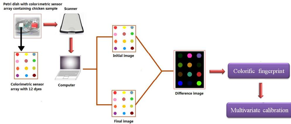
Schematic diagram of E-Nose System based on colorimetric sensor array
