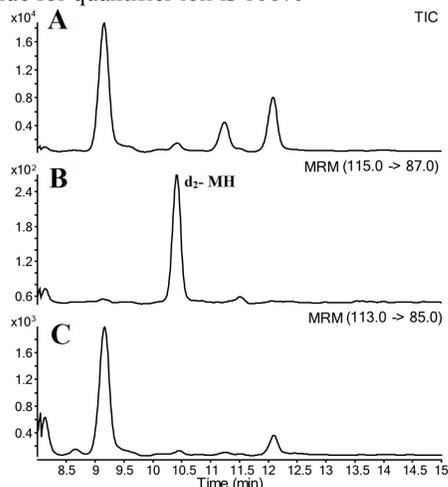
Fig. 1 Chromatograms obtained from blank tobacco sample spiked with the d<sub>2</sub>-MH. (A) Total ion chromatogram. (B) extracted ion chromatogram (m/z 115→87). (C) extracted ion chromatogram (m/z 113→85).
