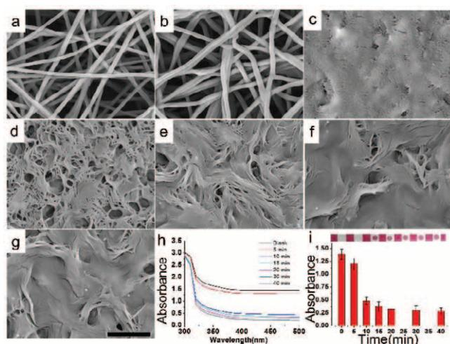
**Figure 3** SEM Images of electrospun fibrous mesh before and after expose to 90.8 % relative humidity for a serial of time (a, 0; b, 5; c, 10; d, 15; e, 20; f, 30; g, 40 min). All images have same magnification and the scale bar is 10 micron; UV-vis spectra (h) and absorbance (i) of electrospun fibrous mesh before and after expose to of 90.8% relative humidity for a serial of time. Error bar represented standard deviation ( $n=3$ ). Insert image in (i) represents the photo of fibrous mesh.
