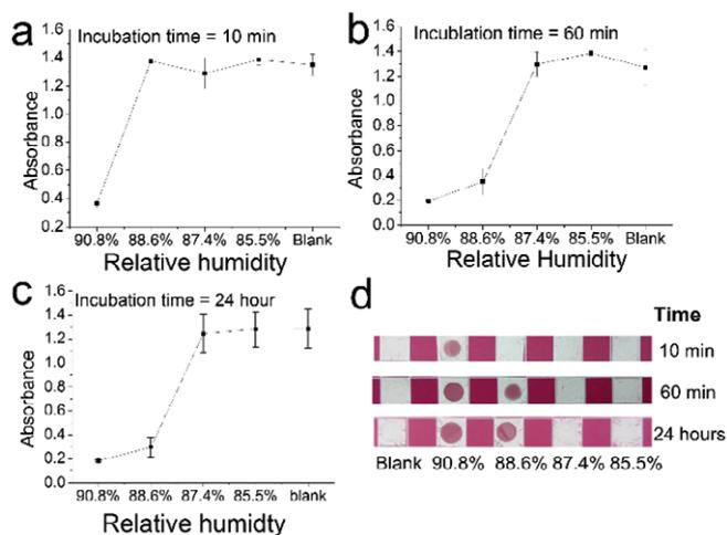
**Figure 4** (a-c) Absorbance of electrospun fibrous mesh expose to different relative humidity condition for 10 min, 60 min, 24 hours. (d) Images of electrospun fibrous mesh exposure to different relative humidity condition for different time. Error bar represented standard deviation ( $n=3$ ).
