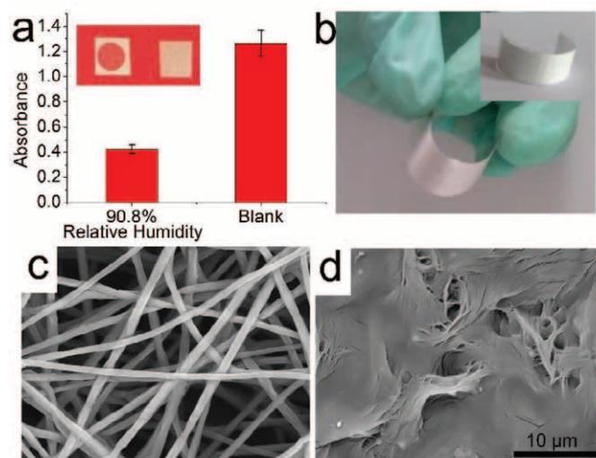
**Figure 2.** (a) Image (insert image) and absorbance of electrospun fibrous mesh before and after exposure to 90.8% relative humidity. Error bar represented standard deviation (n=3). (b) Flexibility of electrospun fibrous mesh on optical clear single-side adhesive film. (c) and (d) SEM image of electrospun fibers before and after exposure to 90.8% relative humidity, respectively. SEM Images (c) and (d) have the same magnification and scale bar is 10 micron.
