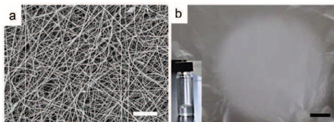
**Figure 1** (a) Morphology of electrospun fibers from 4% w/v PEO polymer solution under scanning electron microscopy. The scale bar is 25 micron. (b) Image of 4%w/v electrospun fibrous mesh on aluminium foil with a scale bar of 2 cm. Insert image is approximate 1 mL of PEO solution in a 4 mL glass vial.
