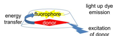
Fig. 1 Illustration of \gamma -cyclodextrin promoted energy transfer, wherein the analyte acts as an energy donor to a high quantum yield fluorophore acceptor.
