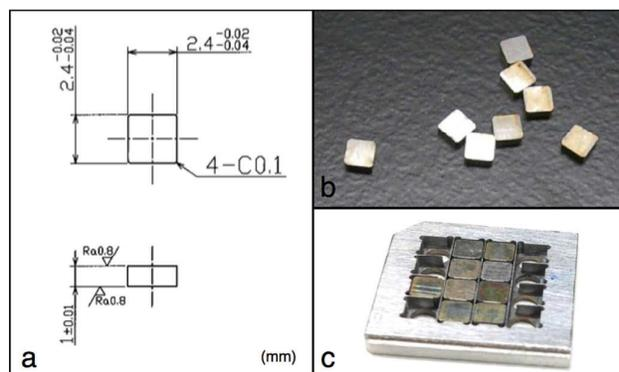
Fig. 2 Microchips and the holding tray. a. Design of the microchip. b. Examples of microchips. c. The holding tray accommodates 16 chips on which a frozen tissue section is overlaid.
