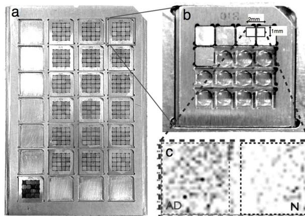
Fig. 3 Custom-made target plates for imaging mass spectrometry of microchips. The target plate (a) holds a 4 x 7 array of holding trays (b) each containing 16 microchips. A 2 x 1 mm area spanning both AD and control sections is analyzed by 58 x 29 dots with 35  $\mu$ m raster step. In (c) is shown an example of preferential binding of a compound to the AD brain section (left side of panel).
