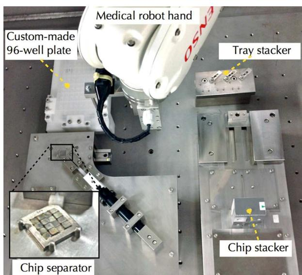
Fig. 1 The robot system. The robot hand was used to transfer microchips according to the following three steps. 1. From the chip stacker to the holding tray on the tray stacker. 2. From chip separator to 96-well plate. 3. From 96-well plate to the tray stacker after immersion in chemical compounds.
