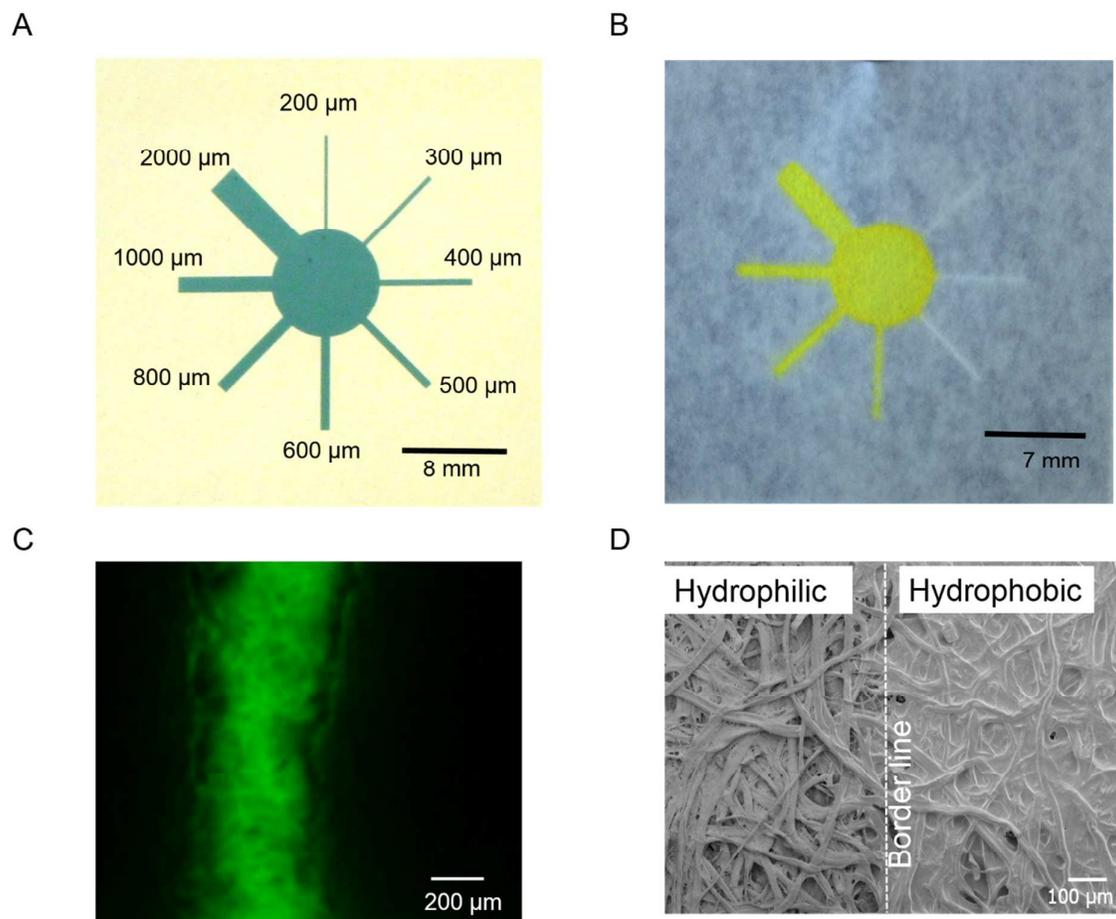
**Figure 2.** Evaluation of different channel widths. A) Patterned screen mesh for printing of different channel widths, B,C) comparison of the printed feature with the patterned screen and tracing the wicking property of them, D) SEM image of the bare (left) and PDMS printed paper (right).
