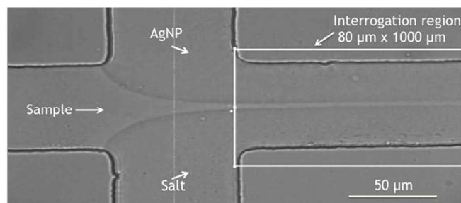
**Figure 1** Flow focusing of the sample at the microfluidic junction. Under laminar flow conditions, the incoming sample stream is hydrodynamically focused between two side-streams, carrying AgNPs and a salt solution respectively, where the species mix by diffusion. As the AgNPs aggregate they become SERS-active, enabling rapid and specific detection of the antibiotic.
