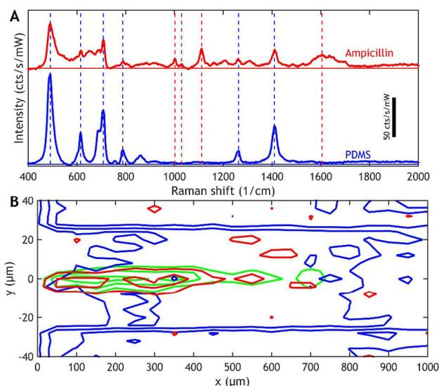
**Figure 2** A) Reference spectra for PDMS and ampicillin (100 ppm in DI water) collected from the channel. B) Contour map of intensities of bands corresponding to the significant chemicals present in the device: blue – PDMS ( $490 \text{ cm}^{-1}$ ), red – ampicillin ( $1115 \text{ cm}^{-1}$ ), and green – AgCl ( $230\text{--}240 \text{ cm}^{-1}$ ).
