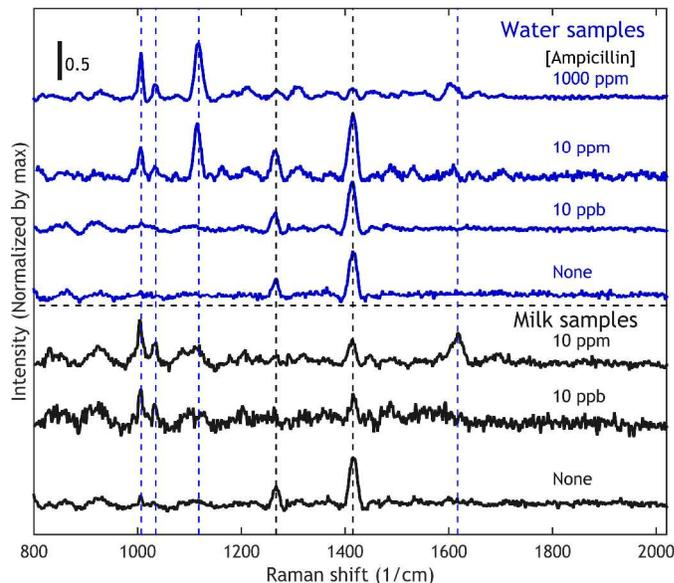
**Figure 3** Average spectra collected. Peaks related with ampicillin were identified from the DI water samples and are marked with the dashed blue lines. These peaks appear in the milk samples spiked with ampicillin, but not in the negative controls. The dashed black lines denote bands at  $1267$  and  $1415\text{ cm}^{-1}$  stemming from the Raman signal of PDMS.
