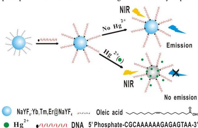
Scheme 1 Schematic illustration of the upconversion biosensor for Hg<sup>2+</sup> ions detection.
