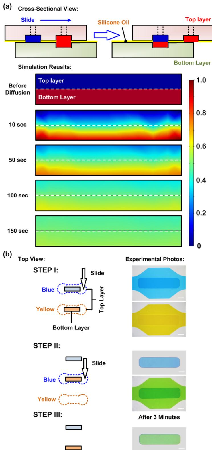
Fig. 2. (a) Schematic and the numerical simulation results of the diffusion between the wells located on the top and bottom layers after contact. (b) The experimental photos of the diffusion between the wells after sliding the top layer for contact. Scale bars are  $500\ \mu\text{m}$
