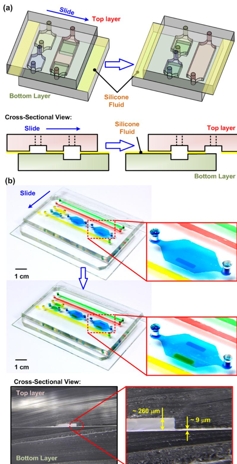
Fig. 1. (a) Schematic and operation of the PDMS SlipChip. (b) Photos of the fabricated PDMS SlipChip with different microfluidic channel arrangements after sliding. The cross-sectional microscopic images show the thickness of the sandwiched Si-Fluid layer is approximately 9  $\mu\text{m}$ .
