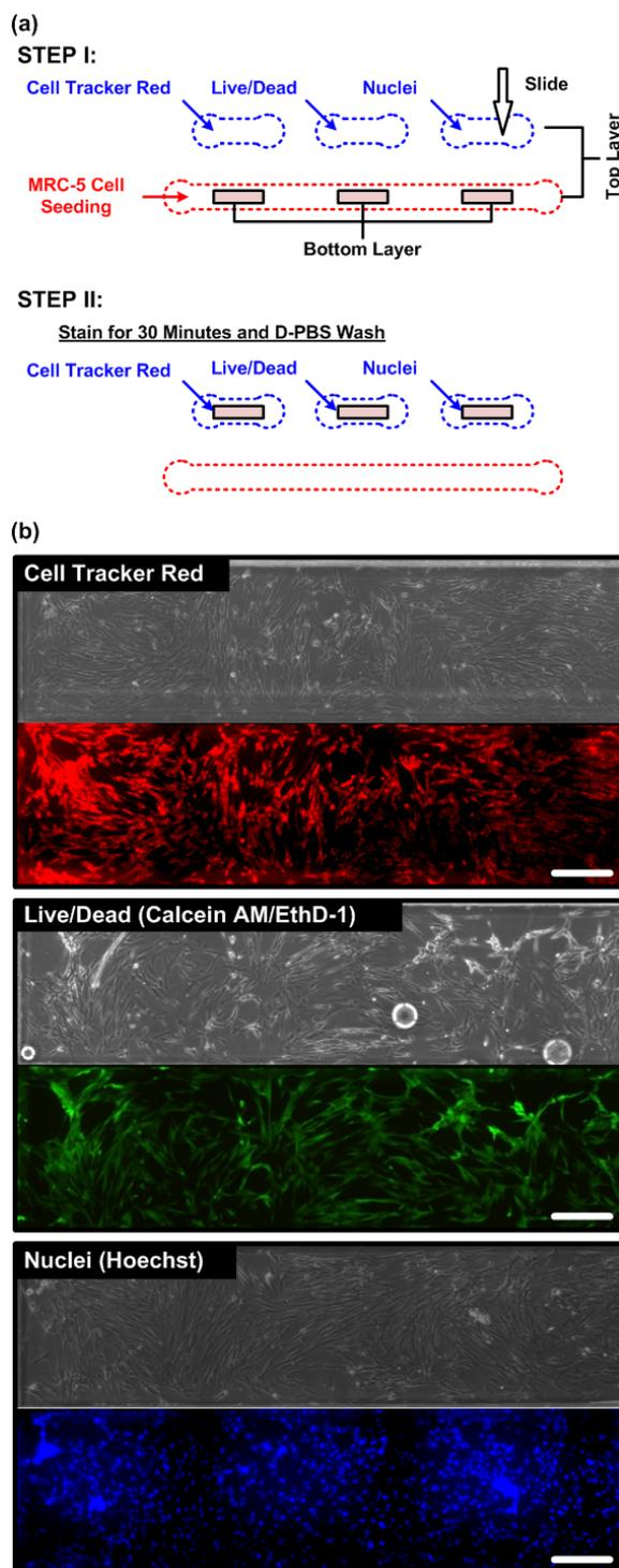
Fig. 5. (a) Operation procedure and the device layout for multiple treatment assays using the PDMS SlipChip. (b) MRC-5 cells located in three different wells are simultaneously stained by Cell Tracker Red, Live/Dead (Calcein AM/EthD-1) and nuclei (Hoechst), respectively. Scale bars are 200  $\mu\text{m}$ . The zoomed-in brightfield phase images of the cells are shown in Supporting Information (Fig. S3).
