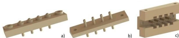
Figure 4 - Fluidic interconnections. a) Tube to chip interconnections, b) Tube to tube interconnections and c) Brackets for fastening the tube to tube interconnections to the tubing.
