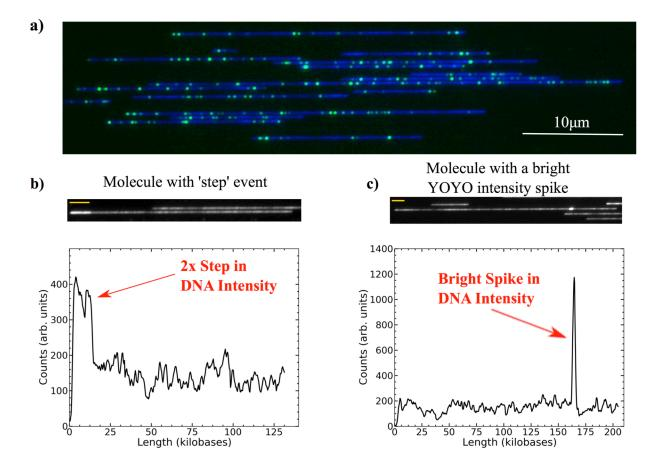
Figure 1 Example of long DNA stretched in nanochannels. (a) A composite image in false color with Nt.BspQI nicks in green, individual long DNA molecule backbones in blue. (b) An image with corresponding YOYO backbone intensity trace of a 'step' event. c) An image and corresponding YOYO intensity trace of a molecule with a small but bright spike in the YOYO intensity. The yellow bars in the molecule images in (b) and (c) correspond to  $4\mu$ m.
