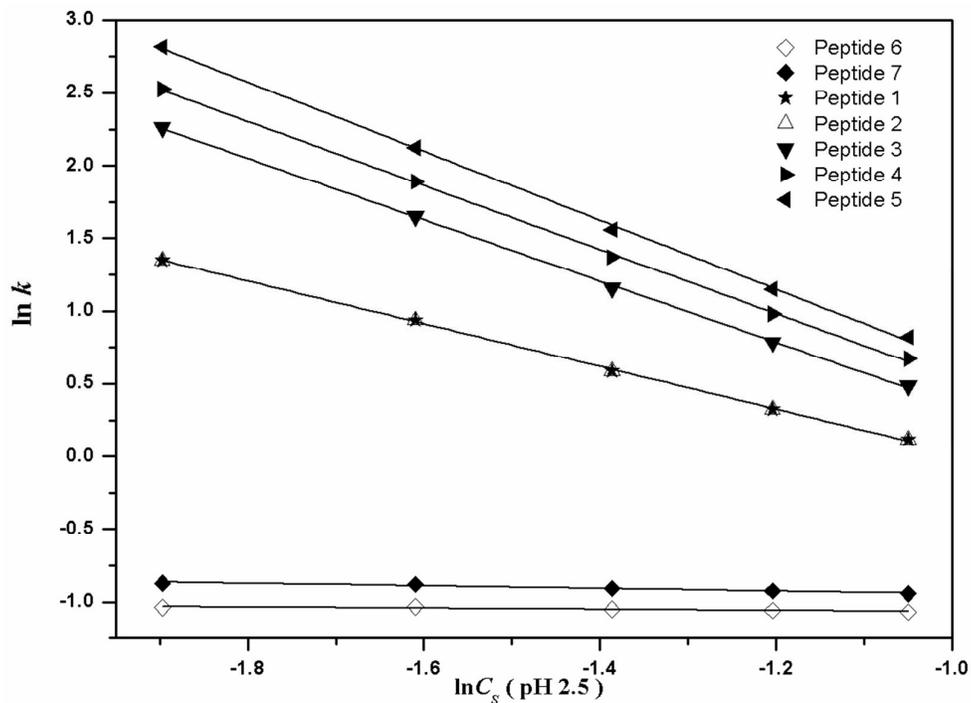
**Fig.3** Plots between logarithms of the retention factor ( $\ln k$ ) versus  $\text{NaClO}_4$  concentration ( $\ln C_s$ ) on the MEX column (250 mm $\times$ 4.6 mm i.d., 10  $\mu\text{m}$ ) at pH 2.5.  $\text{NaClO}_4$  concentrations were 15%, 20%, 25%, 30% and 35%, respectively (150 mM, 200 mM, 250 mM, 300 mM and 350 mM). Conditions: 25% ACN; 10 mM TEAP; flow rate: 1.0 mL/min; column temperature: 30°C; wavelength: 214 nm.
