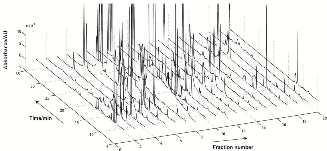
**Fig.7** 3D Chromatograms of 2D-MEX $\times$ C18 system, *x-axis* was the number of fractions, *y-axis* was retention times of peptides in the second dimension, *z-axis* was absorbance responses.
