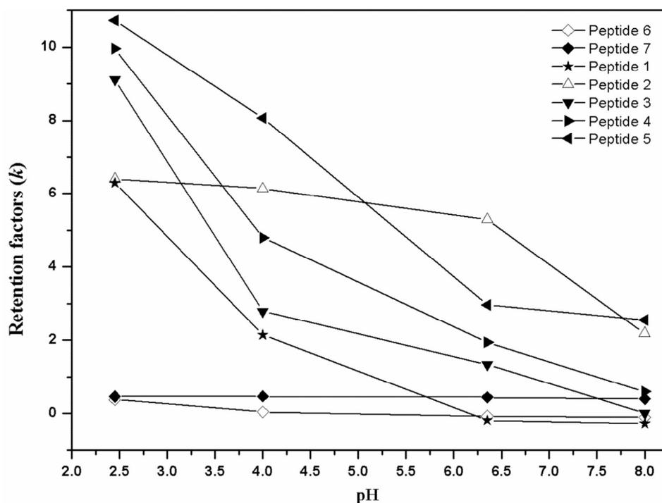
**Fig.5** Plots of peptides' retention factors ( $k$ ) on the MEX column (250 mm×4.6 mm i.d., 10  $\mu$ m) against eluent pH (2.5, 4.0, 6.3 and 8.0). Conditions: 25% ACN; 5%-35% NaClO<sub>4</sub> (50 mM to 350 mM) over 35 min; 10 mM TEAP; flow rate: 1.0 mL/min; column temperature: 30°C; wavelength: 214 nm.
