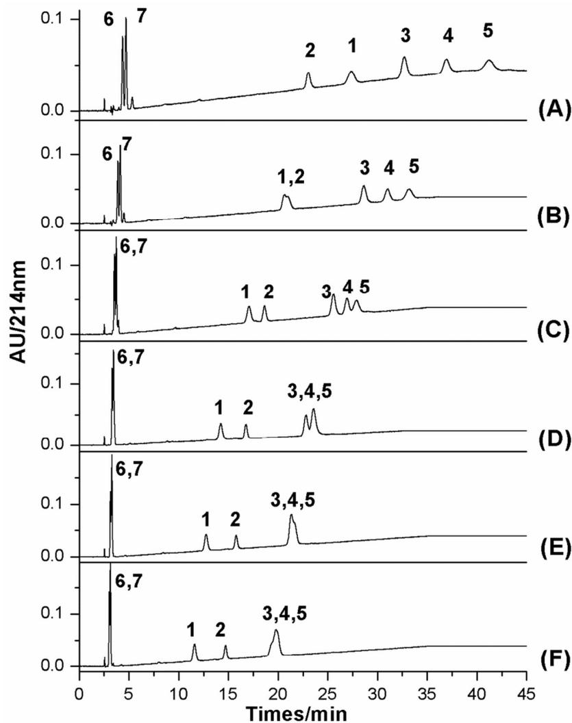
**Fig.1** Chromatograms of seven standard peptides separated on the MEX column (250 mm×4.6 mm i.d., 10 μm) under the different ACN concentration respectively: (A) 20%; (B) 25%; (C) 30%; (D) 35%; (E) 40%; (F) 45%. Seven standard peptides were referred to table 1. Conditions: 5%-35% NaClO<sub>4</sub> (50 mM to 350 mM) over 35 min; 10 mM TEAP, pH 2.5; flow rate: 1.0 mL/min; column temperature: 30°C; wavelength: 214 nm.
