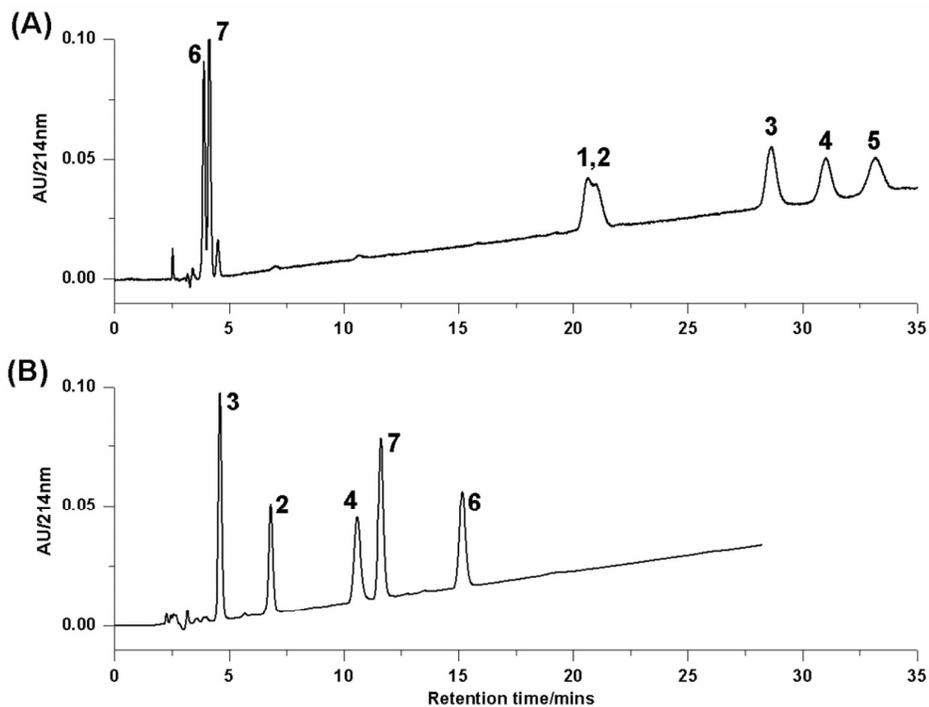
**Fig.2** Chromatograms of seven standard peptides separated on the MEX column (A) and C18 column (B), peptide 1 and 5 were not eluted from C18 column within 35 min. Conditions: 25% ACN; 5%-35% NaClO<sub>4</sub> (50 mM to 350 mM) over 35 min; 10% TEAP (10 mM, pH 2.5); flow rate: 1.0 mL/min; column temperature: 30°C; wavelength: 214 nm.
