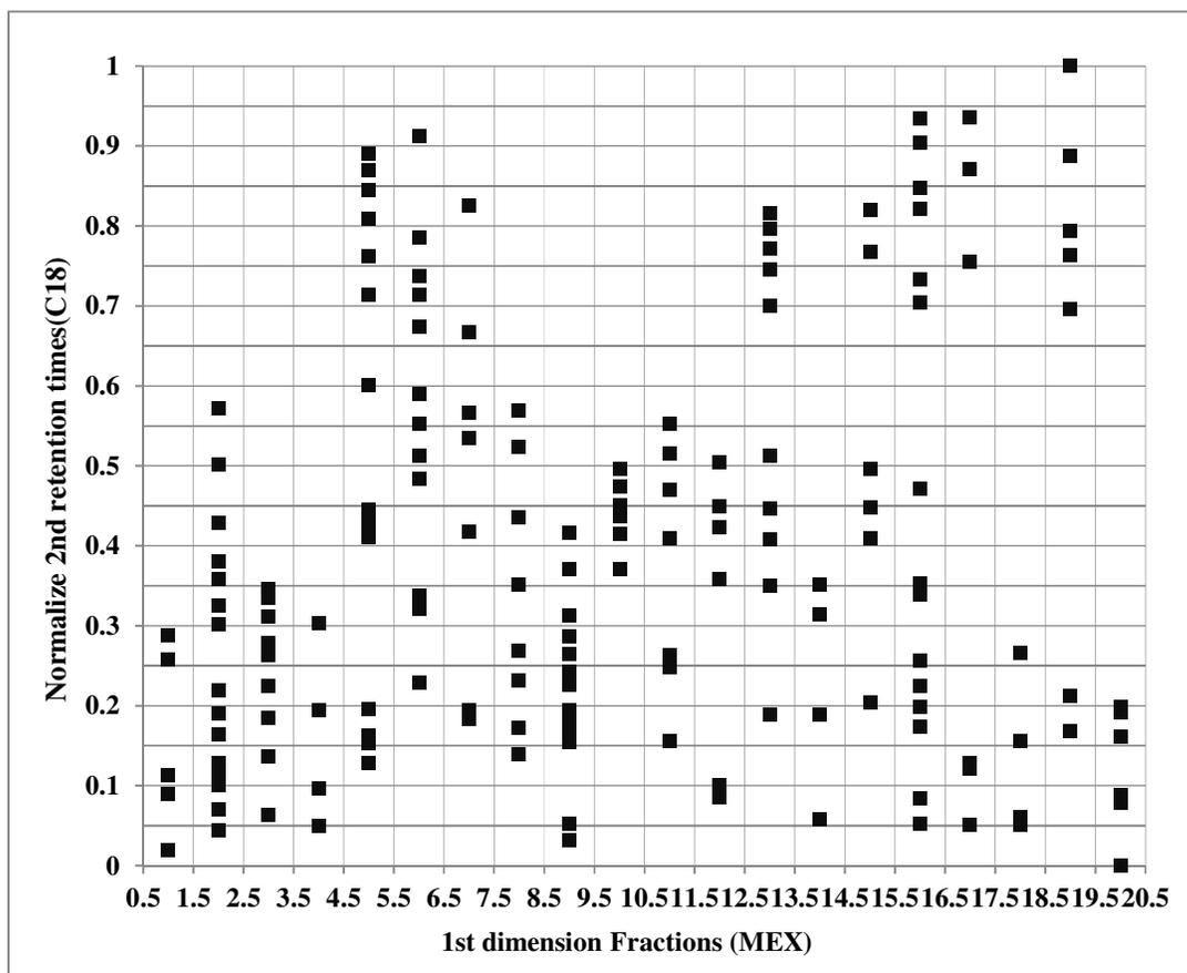
**Fig.9** Normalized retention time plots for 2D-MEX (first dimension) $\times$ C18 (second dimension) in separation of scorpion venom peptides.
