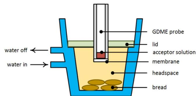
Figure 1 – Extracting scheme. The bread sample was placed inside a thermostatic chamber, a doubled wall glass vessel whose temperature was controlled by a circulating water bath, a poly(methyl methacrylate) lid seals the headspace; the GDME probe with a hydrophobic membrane containing a small volume of acceptor solution is suspended inside.
