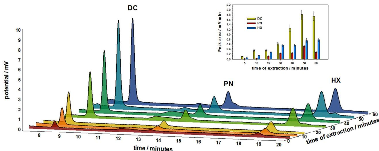
Figure 4 – Chromatograms of several extractions with different extraction times, tested times ranged from 5 minutes up to 1 hour, extractions were performed on 5 g of a bread sample with an aliquot of 100  $\mu\text{L}$  of a solution with 15  $\text{mg L}^{-1}$  of DC, PN and HX. Inlay chromatographic peak area variation with time.
