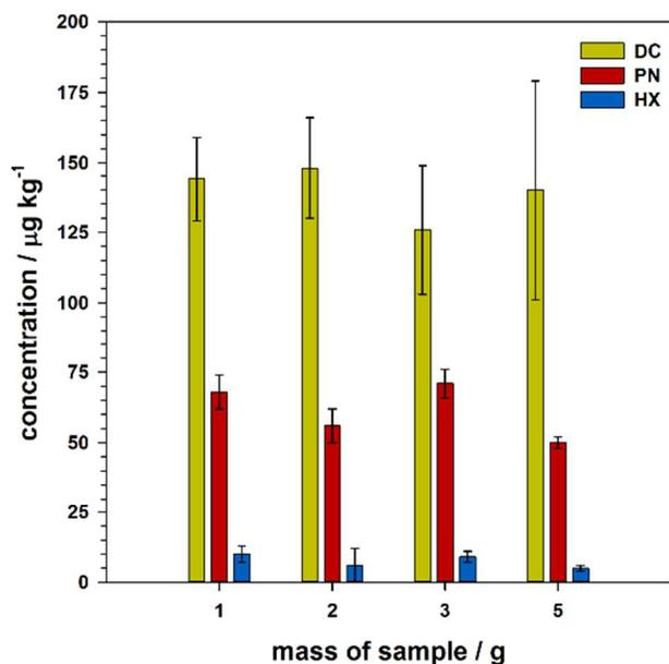
Figure 5 – Determination of DC, PN and HX in a sample of bread using different quantities of sample. For its determination all the standard addition curves had an  $r^2 \geq 0.9$ .
