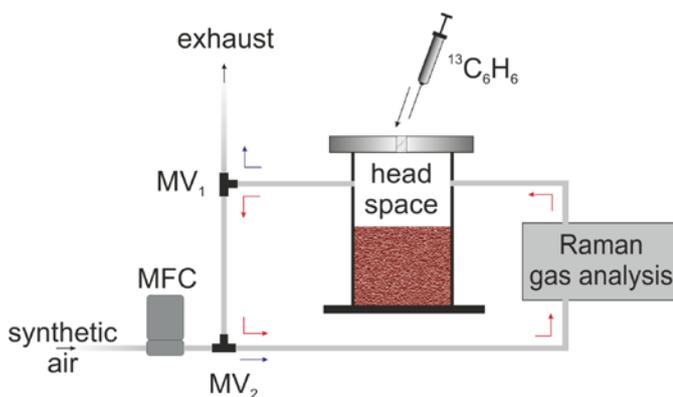
**Figure 2:** Schematic diagram of the experimental setup. Gas flow during rate measurement and flushing indicated by red and blue arrows, respectively. All gas rates were determined within the closable inner cycle, comprising the soil
