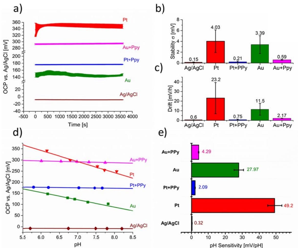
**Fig. 3** Open circuit potential (OCP) measurements of electrode stability and pH sensitivity in a 10mM KCl solution. **(a)** OCP vs. Ag/AgCl as a function of time for each electrode. The bands represent 3 experiments, having the thickness is correlated with repeatability, and fluctuations reflecting stability and drift.
