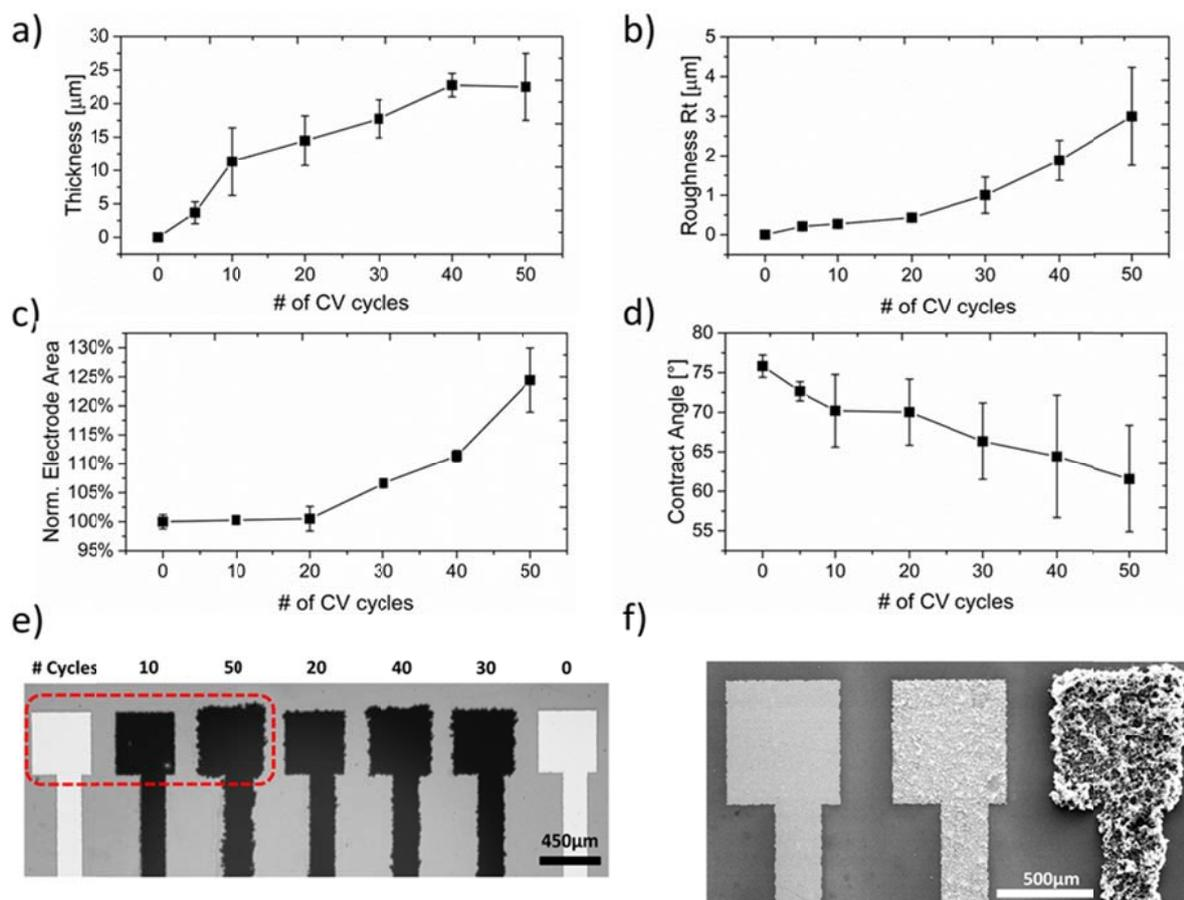
**Fig. 2** Characterization of the deposited PPy film. **(a)** Film thickness, **(b)** Profilometry total roughness (Rt), **(c)** Normalized area of the electrode, and **(d)** contact angle, as a function of the CV deposition cycles. **(e)** Optical image of square electrode array with different numbers of deposition cycles. **(f)** Scanning electron microscopy image of electrodes in the left side of the array presenting 0, 10, and 50 deposition cycles.
