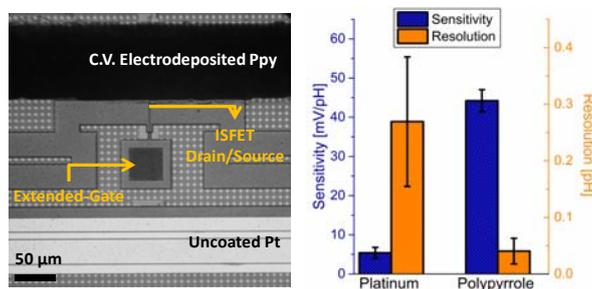
Polypyrrole was deposited on metal electrodes with a cyclic voltammetry process to form robust on-chip quasi-reference electrodes. ISFETs operated with these electrodes are more sensitive and achieve better resolution.
