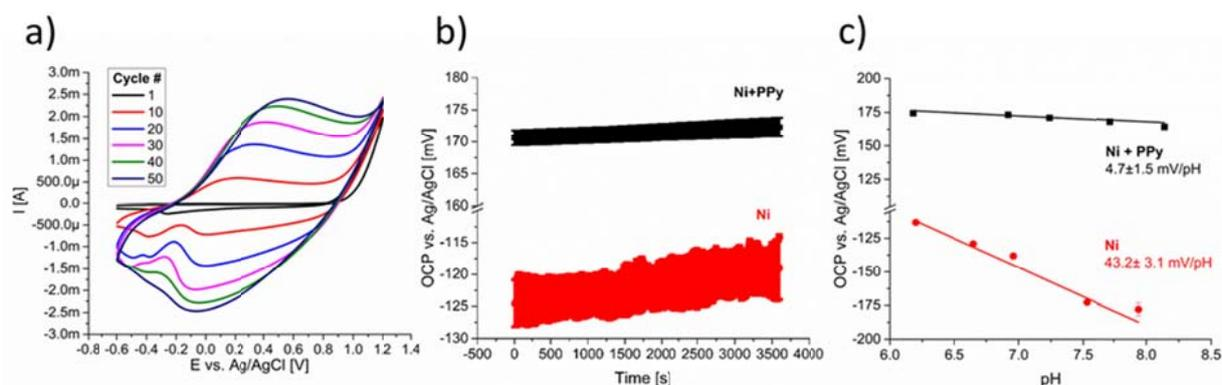
**Fig. 4** Polymerization of PPy on nickel electrodes and electrical performance evaluation. **(a)** CV deposition of PPy film on nickel microelectrodes. **(b)** Bands of OCP stability as a function of time for nickel with and without the PPy layer. **(c)** OCP vs. electrolyte pH to assess pH sensitivity of nickel and nickel+PPy electrodes.
