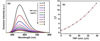
95 Fig. 6 (a) Photoluminescence spectra of complex 4 in acetonitrile-water (v/v = 1: 9) mixtures containing different amounts of TNP. (b) Corresponding Stern–Volmer plots of TNP.
