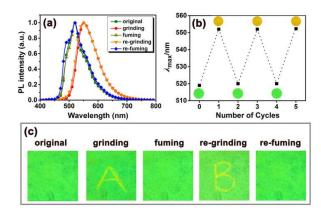
Fig. 4 (a) Emission spectra of complex 4 in various states at room temperature. (b) Maximum emission wavelength change *versus* repeating cycles. (c) Photographs of the reversible writing/erasing cycle using ss complex 4 as medium.
