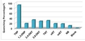
Fig. 7 Quenching percentage obtained for different analytes (9 ppm).
