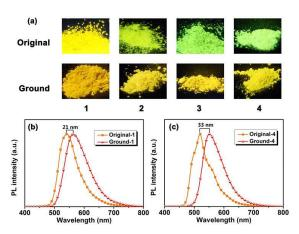
Fig. 3 (a) Photographs of complexes 1–4 taken under UV illumination (365 nm). Emission spectra of complexes 1 (b) and 4 (c) in the solid states at room temperature, respectively.
