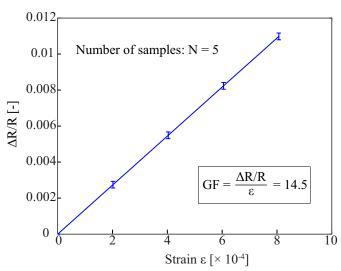
**Fig. 3** The relationship between the relative resistance change of nc-SiC and applied strains.
