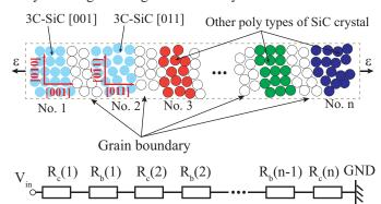
**Fig. 4** An one dimensional (1-D) model of the crystalline structure of nc-SiC which contains a large number of crystalline SiC grains and grain-boundary.
