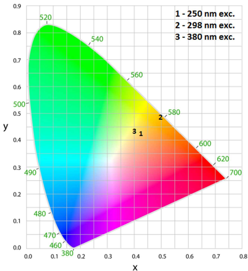
Figure 9. CIE color coordinates diagram presenting the approximate coordinates when Dpdp-ePMO-Eu(tta) 3 sample is excited at different wavelengths: 250 nm, 298 nm, and 380 nm. A change in color of the emitted light at different excitation wavelengths can be observed (CIE coordinates for other excitation wavelengths have been omitted for clarity).
