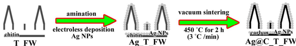
Fig. 1. Schematic representation of the procedure of fabricating the Ag@C_T_FW by electroless deposition and carbonization.
