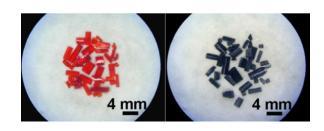
Figure 2. Photos of the red crystals of TiO-L and the blackened crystals.
