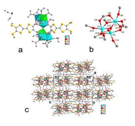
**Figure 1.** (a) Molecular structure of  $[Ti_6O_3(L)_2(O^iPr)_{14}]$ . (b) Enlarged view of the  $Ti_3O_{13}$  cluster; isopropanol groups are omitted for clarity. (c) Molecular packing of TiO-L viewed along the *c* axis.
