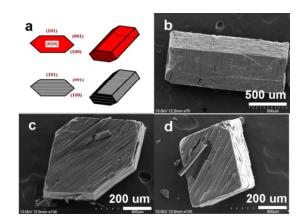
Figure 3. (a) Schematic drawing showing the crystal faces and the cracking texture of the single blackened crystal. SEM images of (b) a small crystal; (c) floor-board-like plates observed on (010) face; (d) disappearing of (101) face viewed along a axis.
