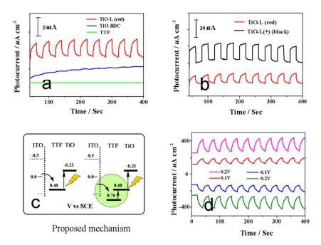
Figure 6. Photocurrent responses in the presence of a  $0.1 \text{ mol} \cdot L^{-1} \text{ Na}_2 \text{SO}_4$  aqueous solution with -0.5 V applied potential of (a) TiO-L, TiO-BDC, TTF and (b) TiO-L and TiO-L(+). (c) Proposed mechanism of the photocurrent responses of TiO-L (left) and TiO-L(+) (right). (d) Photocurrent responses of black crystal TiO-L(+) measured as Schottky-type devices at different bias potentials.
