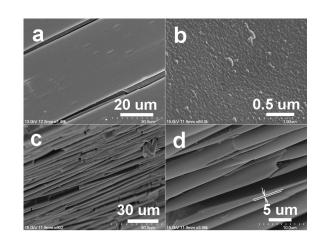
**Figure 4.** SEM images of the morphologies of the blackened crystal: (a, b) surfaces of the plates; (c, d) side views of the plates showing the layered structure.
