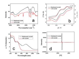
**Figure 5.** (a) FTIR spectra; (b) Solid state cyclic voltammogram in  $CH_3CN$  (0.1 mol·L<sup>-1</sup> Bu<sub>4</sub>NClO<sub>4</sub>, 100 mV s<sup>-1</sup>); (c) UV-vis-NIR absorption spectra; (d) ESR spectra recorded at 110 K of the red crystals TiO-L and the blackened crystals.
