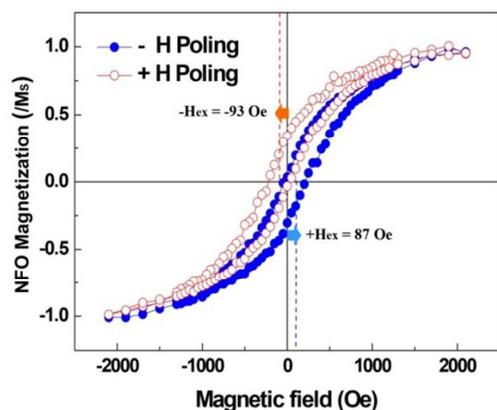
**Fig. 3** Minor hysteresis loops extracted from the major hysteresis curve for magnetic fields in between +2 kOe and -2 kOe. The magnetization attributed to the CFO layer was subtracted from the data, and then normalized to the saturated magnetization. The magnetic shifts in these exchange biased loops are -93 Oe and +87 Oe, respectively, with respect to magnetic poling directions.
