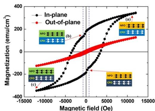
**Fig. 2** Room-temperature magnetization-field hysteresis curves of the two magnetic layers measured along in-plane and out-of-plane directions. It shows the magnetic easy axis with in-plane direction. Abrupt change in magnetization near a zero magnetic field (blue dot-lines) arises from the rotation of spins in the NFO layer with keeping the spins in the CFO layer fixed. Schematic spin configurations for different states of a hysteresis are depicted in insets
