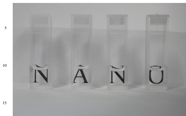
Fig. 1 Picture of \text{Eu}^{3+} - and \text{Tb}^{3+} -doped \text{CaF}_2 (from left to right: \text{CaF}_2:\text{Tb}10 , mixture of 52% of \text{CaF}_2:\text{Tb}10 + 48% of \text{CaF}_2:\text{Eu}10 , \text{CaF}_2:\text{Tb}5.2, \text{Eu}4.8 and \text{CaF}_2:\text{Eu}10 ).
