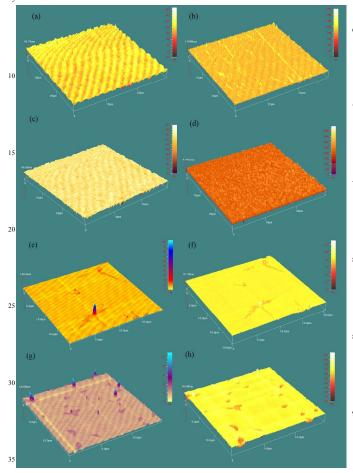
Figure 8. AFM surface topography (Left) and corresponding phase (Right) images of pristine PFO (a-d) and PFO/PNDIT-alt-DTP containing 95:5 wt.% copolymer (e-f) thin films : (a), (b), <sup>40</sup> (e) and (f) for as spun film and (c), (d), (g) and (h) for films annealed at 120 °C. Note that PNDIT-alt-DTP chains are molecularly dispersed in the PFO matrix due to the low content.
