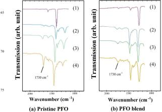
Figure 9. FTIR spectra of polymer films. a) PFO film, b) <sup>80</sup> PFO/PNDIT-alt-DTP containing 95:5 wt. % blend film, before (1) and after annealing in the oven of 40°C for 5 min (2), 30 min (3), and 60 min (4). The >C=O stretching mode at ~1730 cm<sup>-1</sup> is changed in (a) but is almost unchanged in (b). All data points used to create the plots were averaged over four trials.
