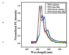
Figure 4. Normalized Fluorescence spectra of pristine PFO 40 solution, spin-cast film annealed at 60°C in air and PFO blend with 5 wt. % PNDIT-alt-DTP.
