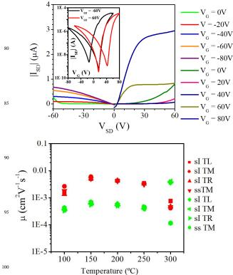
Figure 3. a) Typical transistor output and transfer characteristics of a PNDIT-alt-DTP transistor annealed at 150 °C, with transfer curve in the inset. Mobilities were determined to be 0.07 <sup>105</sup> cm<sup>2</sup>V<sup>-1</sup>s<sup>-1</sup> for n-type transport and 0.006cm<sup>2</sup>V<sup>-1</sup>s<sup>-1</sup> for p-type transport. b) Transistor mobilities as a function of annealing temperature for PNDIT-alt-DTP for n-type transport (red) and ptype transport (green).
