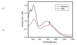
Figure 1. UV-vis-NIR absorption spectra of PNDIT-alt-DTP in <sup>35</sup> CHCl<sub>3</sub> solution and thin film on glass substrate.
