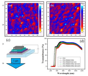
Figure 6. (a) Phase-imaging tapping-mode AFM of 35 PEDOT:PSS:GO composite at room temperature; and (b) Phase alignment after thermal treatment at 120°C (1.4µm x 1.4µm region); (c) Scheme of the PLED device structure and (d) UV-vis spectra for pure and modified HIL. Transmittance for pure ITO (black) and ITO/PEDOT:PSS (purple) and others modified by 40 different percentages of GO.
