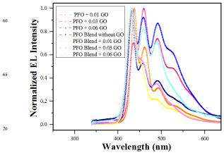
Figure 7. Normalized Electroluminescence of pure PFO PLEDs: ITO/PEDOT:PSS:GO/PFO/Al and PFO blend with 5 wt.% 75 PNDIT-alt-DTP: ITO/PEDOT:PSS:GO/PFO blend/Al. Error bars are 95% confidence intervals for the corrected fluorescence intensity at  $\lambda_{max}$ . All data points used to create the plots were averaged over four trials.
