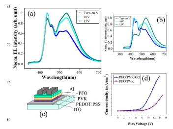
Figure 5. a) Relative EL intensity of device ITO/PEDOT:PSS:GO/PVK/PFO/Al; b) EL intensity of device ITO/PEDOT:PSS/PVK/PFO/Al; c) The cartoon picture shows the so device schematic; d) Current density-Voltage (*J-V*) characteristics of these two PLEDs with: pure PEDOT:PSS and blends with GO. All data points used to create the plots were averaged over four trials.
