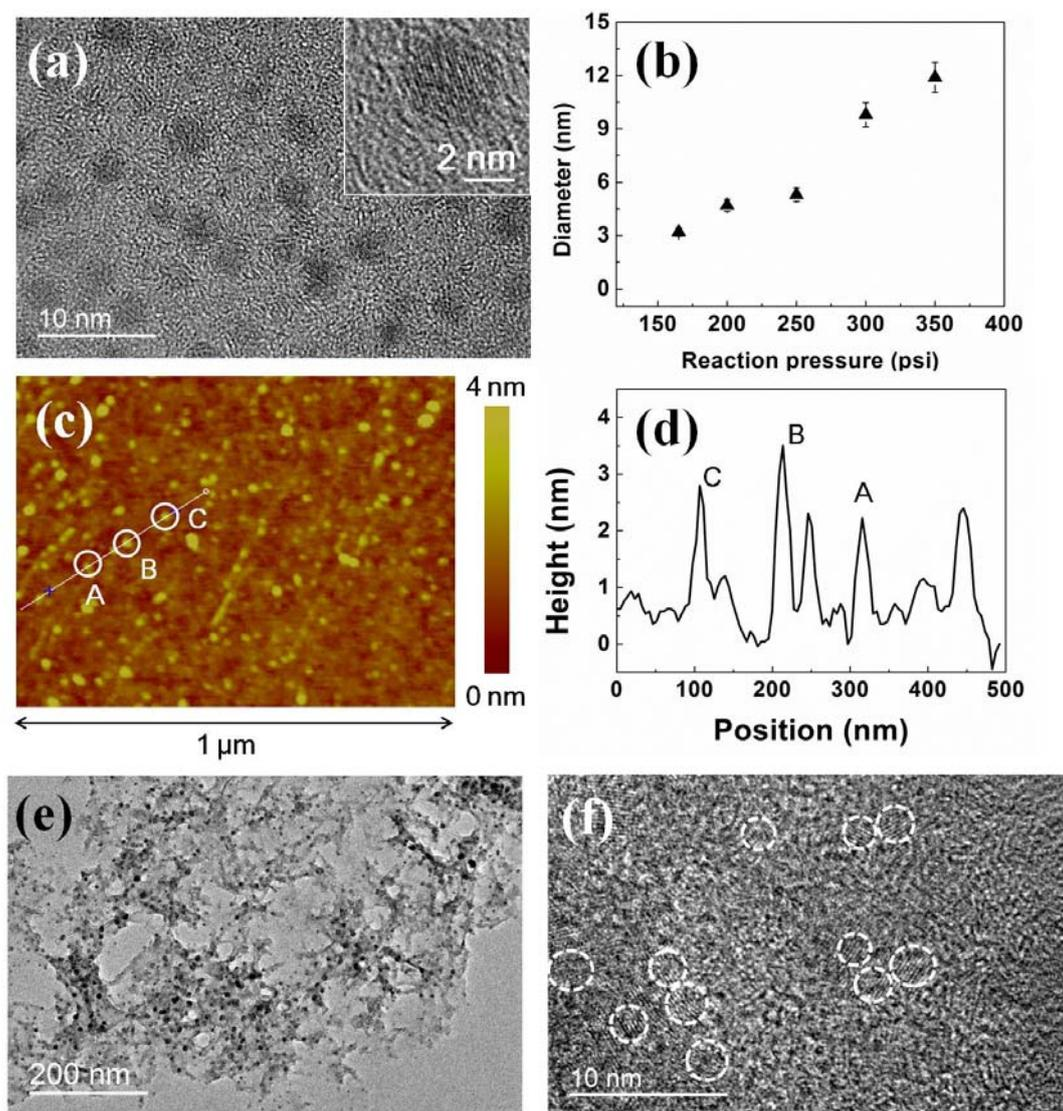
Figure 3 (a) High-resolution TEM image of the GQDs. (b) The diameter of the GQDs for various reaction pressures. (c) AFM image of the GQDs. (d) The height analyses of the GQDs as shown in AFM image (c). (e) and (f) low magnification and High-resolution TEM images of the PANI-GQD composite respectively.
