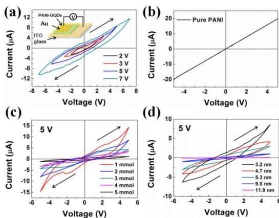
Figure 5 (a) Hysteresis behavior of the Au/PANI-GQD/ITO structure under different voltages. The inset depicts the device structure. (b) Linear relationship of the current-voltage characteristics of PANI. Hysteresis loops measured at (c) various moles of aniline and (d) sizes of the GQDs respectively. All the hysteresis behaviors were measured in clockwise direction with respect to the voltage.
