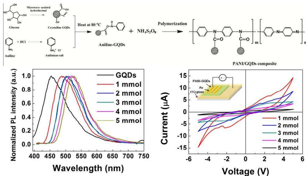
The tunable photoluminescence and transport properties of PANI-GQD composite is reported by adjusting the sizes of the GQDs and the amounts of PANI.
