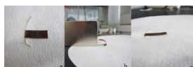
Fig. 3 Bending and stretching movements of free-standing Alg/(PEI-PEG/ \alpha -CD/ \text{Fe}_3\text{O}_4 ) film with changing the placement of permanent magnet.
