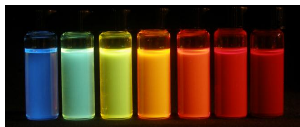
Fig. 1 – Toluene solutions of oleylamine capped Zn 3 N 2 nanocrystals sampled at different reaction times excited with a 365nm lamp
