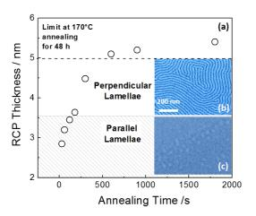
**Fig. 5** Thickness of the RTP grafted films of R58 at 250°C as a function of time. The two thickness widows corresponding to perpendicular and parallel orientations of the lamellae are also indicated. SEM images corresponding to parallel (b) and perpendicular (c) orientation of the lamellae microdomains are reported.
