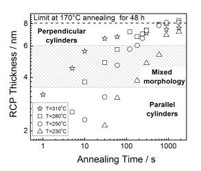
**Fig. 1** Thickness of the RTP grafted films of R62 at 230, 250, 280°C and 310°C as a function of time. The three zones in which the orientation the cylinders is changed (perpendicular cylinders, mixed morphology and parallel cylinders) are also indicated.
