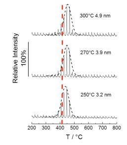
Fig. 9 TGA-GC-MS analysis of styrene for R58 after annealing the thin film in RTP for 1 min at temperatures comprised between 250 and 300°C. The grafted film thickness is reported for each temperature. The dashed red line was added to guide the eyes.
