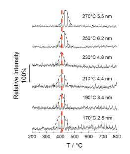
**Fig. 8** TGA-GC-MS analysis of styrene for R58 after annealing the thin film in RTP for 15 min at temperatures comprised between 170 and 300°C. The grafted film thickness is reported for each temperature. The dashed red line was added to guide the eyes.
