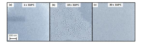
Fig. 4 SEM images of the PS-b-PMMA B70 morphologies obtained on the random copolymer R62 subjected to RTP grafting under various time at 310°C.
