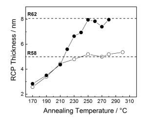
**Fig. 6** Thickness trend for R62 (full symbol) and R58 (open symbol) as a function of the annealing temperature after 15 min annealing time. The dashed lines indicate the limiting thickness for grafting in oven at 170°C annealing for 48 h.
