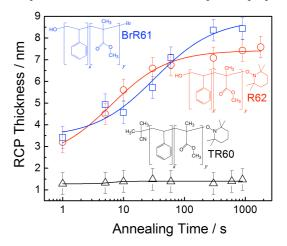
Fig. 2 Thickness of the RTP treated films of R62 (red circles), TR60 (black triangles) and BrR61 (blue squares) at  $310^{\circ}$ C as a function of time.
