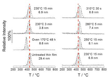
**Fig. 7** TGA-GC-MS analysis of styrene performed on R62 films, featuring different thicknesses and subjected to distinct thermal treatments. The dashed red was added to guide the eyes.
