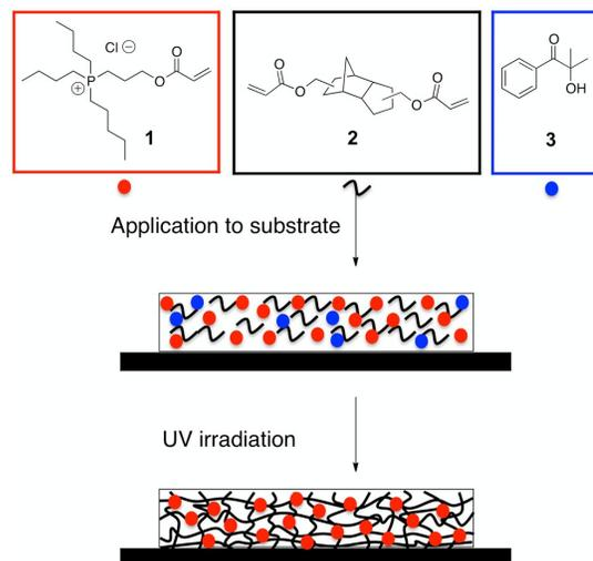
Fig. 1. Schematic showing the coating preparation process.
