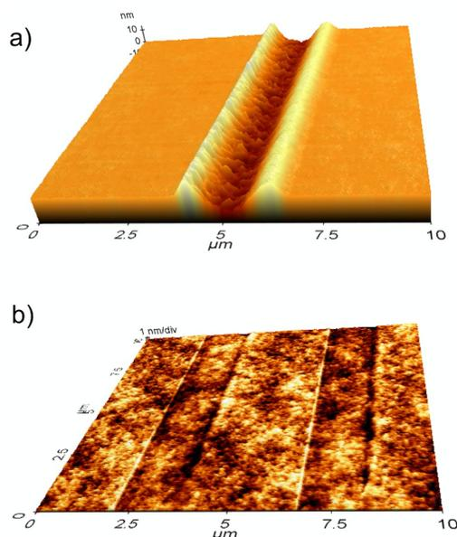
Fig. 2. AFM images following application of a diamond tip surface profiler with a 0.5 mN force to: a) a film cured in air and b) a film cured under N<sub>2</sub>.
