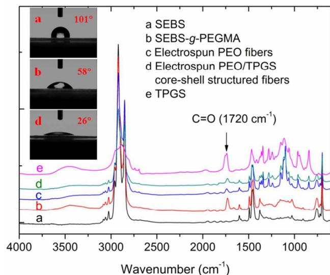
Fig. 2 ATR-FTIR spectra of SEBS, electrospun fiber and TPGS. The insets are the images of water contact angle on the surface of SEBS samples. (a) virgin SEBS, (b) SEBS-g-PEGMA, (c) electrospun PEO fibers, (d) electrospun TPGS / PEO fibers, (e) TPGS.
