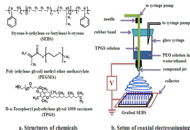
Fig. 1 Chemical structures of substances (a) and setup of coaxial electrospinning for fabrication of nanofibers on the grafted SEBS (b).
