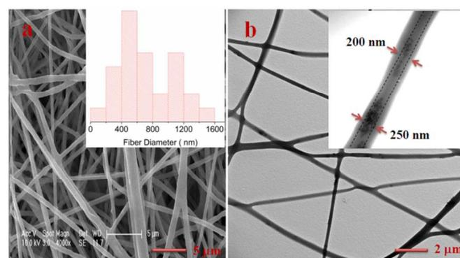
Fig. 3 SEM and TEM images of core-shell structured nanofibers. (a) SEM image of electrospun fibers; (b) TEM images of nanofibers on a copper grid. The inset is the segment of the nanofibers with scattered inner component.
