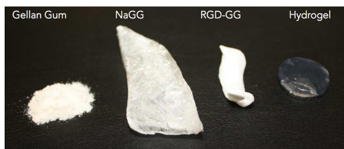
Figure 2: Gellan gum (GG) through each stage of processing. From left to right, as-received (commercial) GG powder, lyophilised NaGG, lyophilised RGD-GG and a 0.9% (w/v) RGD-GG hydrogel.
