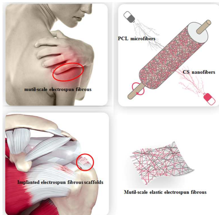
Scheme 1 Illustrations of fabrication of dual scaffolding system composed of PCL microfibers and interspersed CS nanofibers using a stagger-electrospinning process with a rotating metal mandrel for augmentation of RCT tendon-healing.
