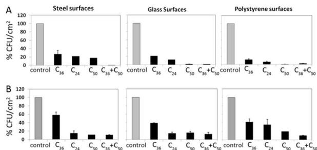
**Fig. 3.** Live bacterial counts on uncoated steel, glass or polystyrene surfaces (control) and on surfaces coated with C<sub>24</sub>F<sub>50</sub>, C<sub>36</sub>H<sub>74</sub>, C<sub>50</sub>H<sub>102</sub> or C<sub>36</sub>H<sub>74</sub>+C<sub>50</sub>H<sub>102</sub>. Biofilms were grown in LB liquid media for 24 h (A) *B. cereus* biofilms, (B) *P. aeruginosa* biofilms.
