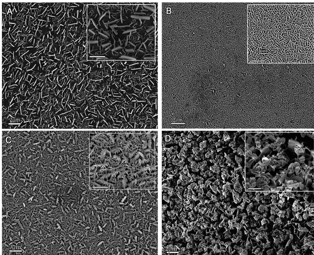
**Fig. 1.** HR-SEM micrographs of 3D crystalline structures thermally evaporated on glass substrates (A)  $C_{36}H_{74}$  (B)  $C_{36}H_{74}+C_{50}H_{102}$ , (C)  $C_{50}H_{102}$  and (D)  $C_{24}F_{50}$ . Insets were acquired at a  $30^\circ$  tilt angle. Scale bar is  $1\ \mu\text{m}$
