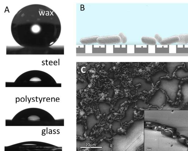
**Fig .6.** (A) optical images of a 7µL water droplet on various substrates, (B) a schematic describing the bacteria-surface interface on a superhydrophobic surface and (C) HRSEM micrograph of *B. cereus* on flat steel substrate.
