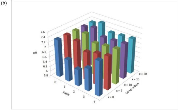
Fig. 13. pH changes of solution during solubility studies of studied glasses in (a) deionised water and (b) tris/HCl buffer
