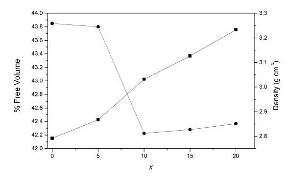
Fig. 3. Compositional variation of density (squares) and % free volume (circles) in the system  $10\text{Na}_2\text{O}:(20 + x/2)\text{ZnO}:(20 + x/2)\text{CaO}:(50 - x)\text{P}_2\text{O}_5$ .
