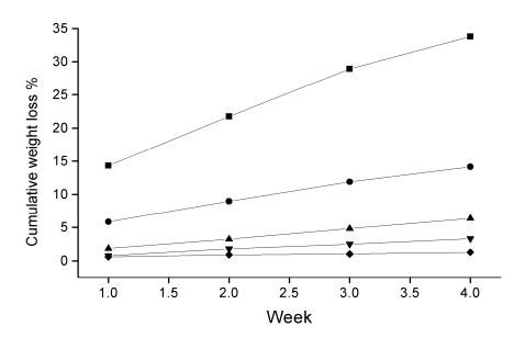
Fig. 14. Cumulative percentage weight loss of glass discs as a function of time in (a) de-ionised water and (b) tris/HCl buffer, showing x = 0 (squares), x = 5 (circles), x = 10 (up triangles), x = 15 (down triangles) and x = 20 (diamonds) compositions.
