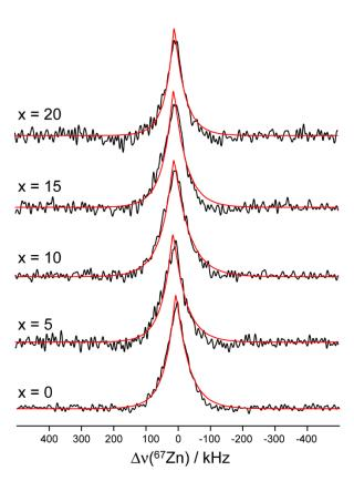
Fig. 8.  $^{67}$ Zn NMR spectra are shown for glasses in the system  $10\text{Na}_2\text{O}:(20 + x/2)\text{ZnO}:(20 + x/2)\text{CaO}:(50 - x)\text{ P}_2\text{O}_5$  (in black) along with their Czjzek simulations. The simulation parameters are listed in Table 4.
