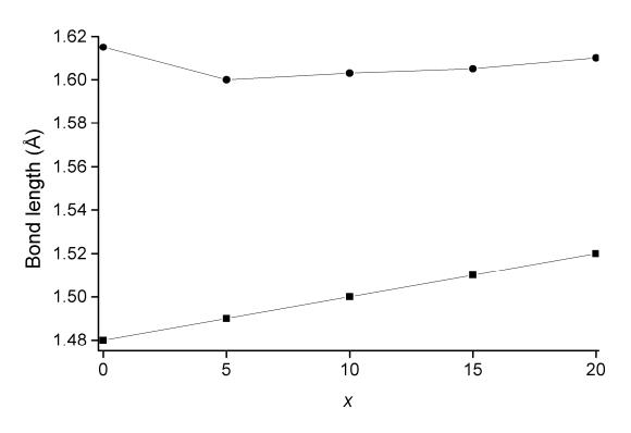
Fig. 12. Compositional variation of P–O bond lengths in glasses in the system  $10\text{Na}_2\text{O}$ :(20 + x/2)ZnO:(20 + x/2)CaO:(50 - x) P<sub>2</sub>O<sub>5</sub>, showing distances to bridging oxygen (P–BO) and non-bridging oxygen (P-NBO) atoms.
