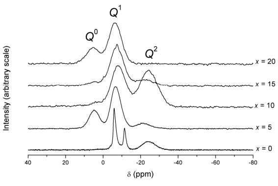
Fig. 16. Isotropic resonances in  $^{31}P$  MAS-NMR spectra of glasses of composition  $10Na_2O-(20 + x/2)ZnO-(20 + x/2)CaO-(50 - x)P_2O_5$  after immersion for 28 days in tris/HCl buffer. Spectra were measured at 21 kHz spinning speed.
