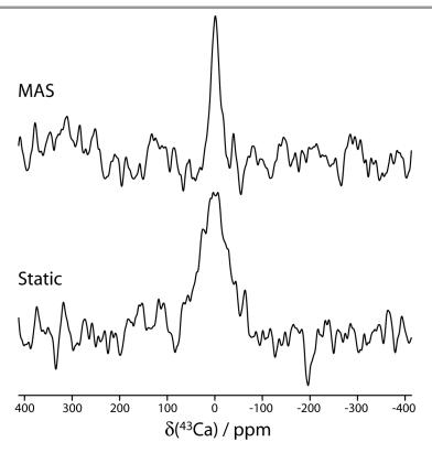
Fig. 9.  $^{43}$ Ca static and MAS-NMR spectra for the x = 15 glass composition.
