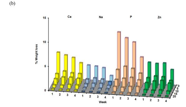
Fig. 17. Ion release profiles for studied glasses immersed in (a) deionised water and (b) tris/HCl buffer. Values are presented as percentage weight loss normalised to the ion content in the parent glass and with respect to the weight in the previous week.
