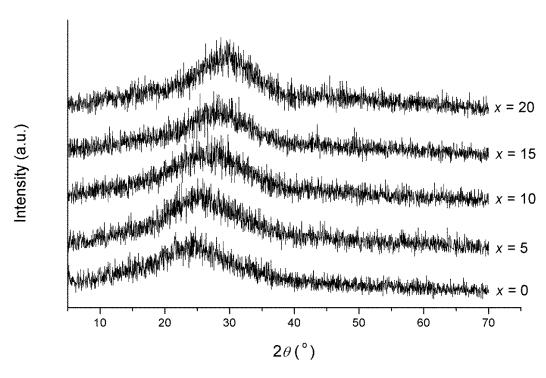
Fig. 1. X-ray diffraction patterns for glasses of composition  $10\text{Na}_2\text{O}:(20 + x/2)\text{ZnO}:(20 + x/2)\text{CaO}:(50 - x)\text{P}_2\text{O}_5$ .
