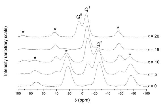
Fig. 5. Isotropic resonances in  $^{31}P$  MAS-NMR spectra of glasses of composition  $10Na_2O:(20 + x/2)ZnO:(20 + x/2)CaO:(50 - x)P_2O_5$  measured at 12 kHz spinning speed.
