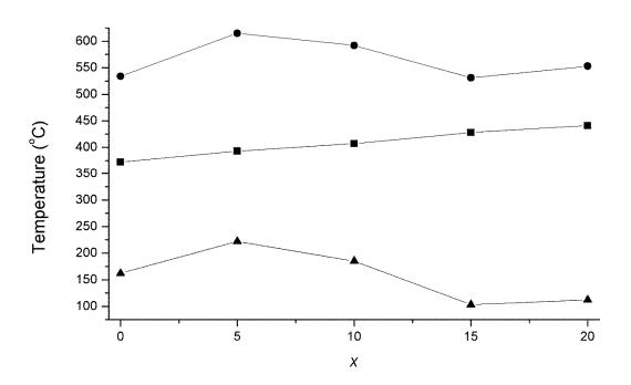
Fig. 2. Compositional variation of  $T_c$  (circles),  $T_g$  (squares) and  $T_c - T_g$  (triangles) for glass compositions in the system  $10\text{Na}_2\text{O}:(20+x/2)\text{ZnO}:(20+x/2)\text{CaO}:(50-x)\text{P}_2\text{O}_5$ . Lines are a guide to the eye.
