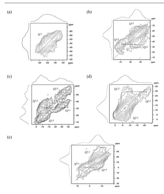
Fig. 6.  $^{31}$ P- $^{31}$ P DQ MAS-NMR spectra of studied glass compositions; (a) x = 0, (b) x = 5, (c) x = 10, (d) x = 15 and (e) x = 20. The lowest contour levels are set to 10% and levels increase in steps of 10%.
