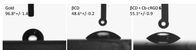
Figure 2. Water contact angle values for gold, \beta CD monolayer and \beta CD complexed with Cb-cRGD 6 ( n=4 ), with a representative picture. A high WCA angle value indicates a hydrophobic surface.
