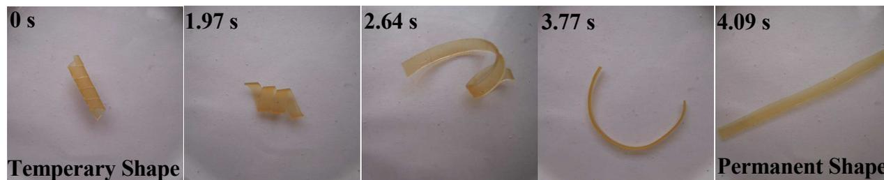
**Fig. 8** Transition from the temporary spiral shape to the permanent linear shape for PBISI-2 SMP. The samples were cured with 0.4 phr of DCP and the recovery process was recorded after heating the samples to  $T_m+10^\circ\text{C}$ .
