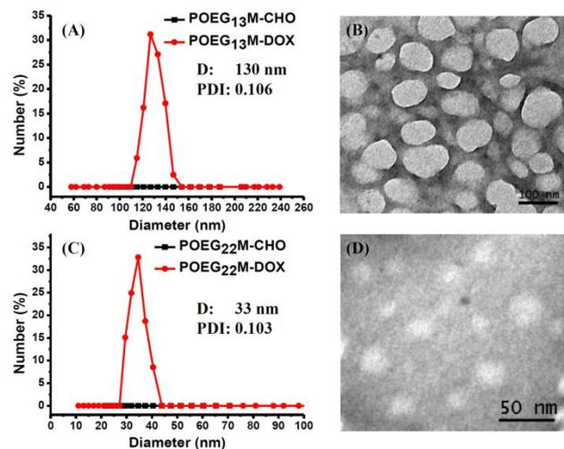
**Fig. 4** Particle size, distribution of POEG<sub>13</sub>M-DOX micelles (A) and POEG<sub>22</sub>M-DOX micelles (C) measured by DLS; TEM images of POEG<sub>13</sub>M-DOX micelles (B) and POEG<sub>22</sub>M-DOX micelles (D).
